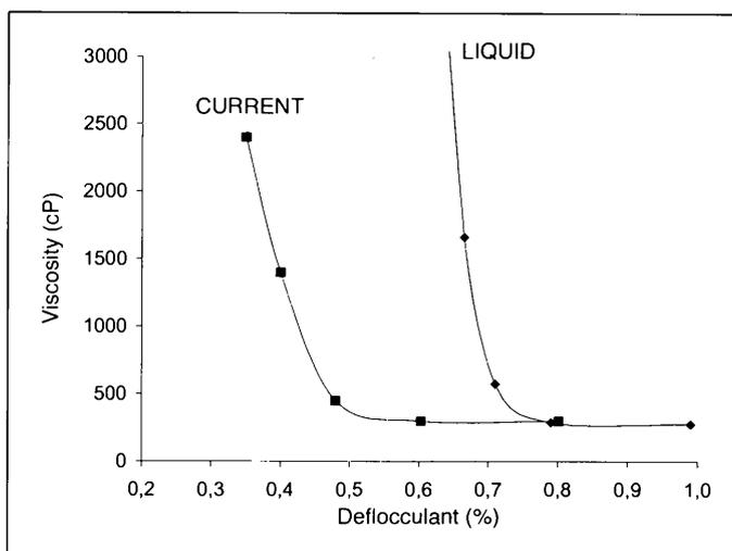
Figure 2. Variation of apparent viscosity of a porous redware wall tile composition suspension with deflocculant percentage.
