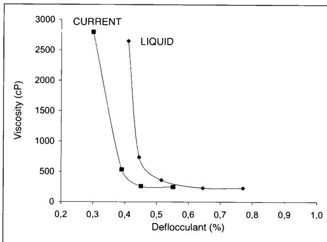
Figure 1. Variation of apparent viscosity of a white stoneware floor tile composition suspension with deflocculant percentage.
