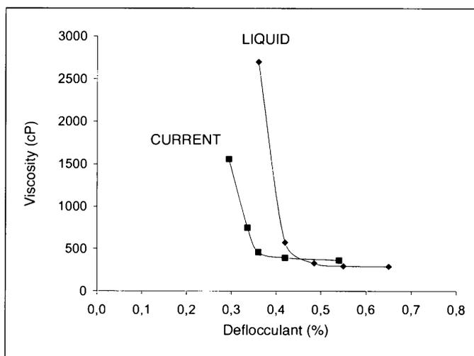
Figure 3. Variation of apparent viscosity of a porcelain tile composition suspension with deflocculant percentage.
