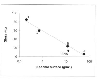
Figure 1. Relation between gloss and alumina specific surface..
