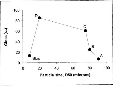
Figure 2. Relation between gloss and mean alumina particle size.
