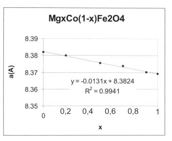
*Figure 1. Variation of the spinel unit cell with x.*
