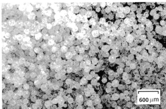
Figure 8. Granules treated in the lengthened laboratory reactor at 1700°C.
