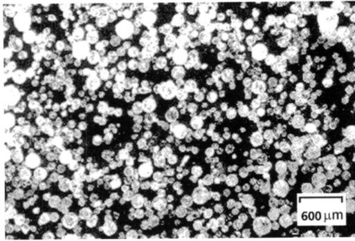
Figure 6. Granules treated in the laboratory reactor at 1700°C.
