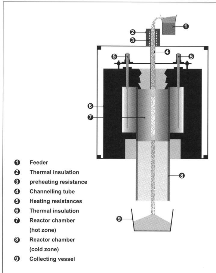
Figure 1. Schematic illustration of the laboratory reactor.
