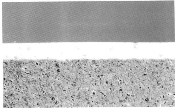
*Figure 13. Appearance of the cross section of the glaze obtained with the spheroidised frit of Figures 10 and 11.*
