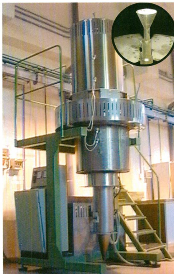
Figure 3. Assembly of the pilot-scale dilute-phase reactor.
