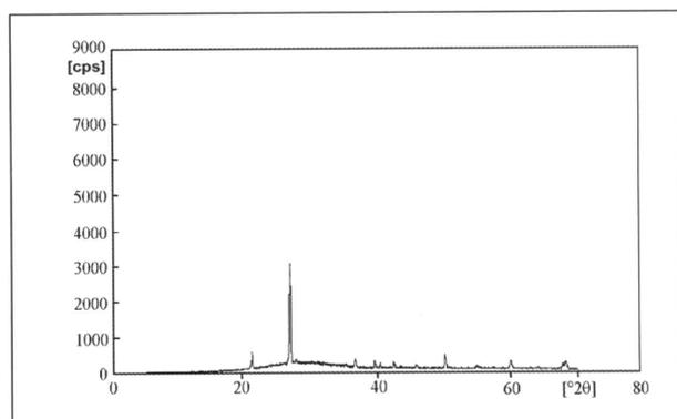
Figure 9. Diffractogram of the granules treated in the laboratory reactor with a lengthened chamber at 1700°C.
