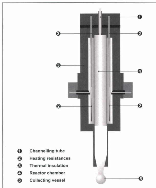
Figure 2. Schematic of the pilot-scale reactor.
