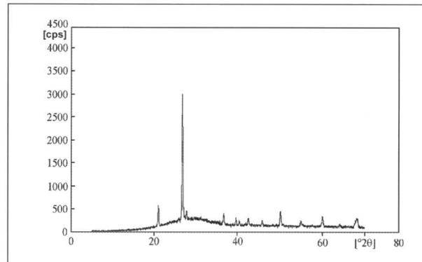
Figure 5. Diffractogram of the granules treated in the laboratory reactor at 1500°C (D<200 µm).
