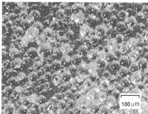
Figure 16. Appearance of the product obtained in the pilot-scale reactor. Fine fraction ( $D < 100 \mu\text{m}$ ).
