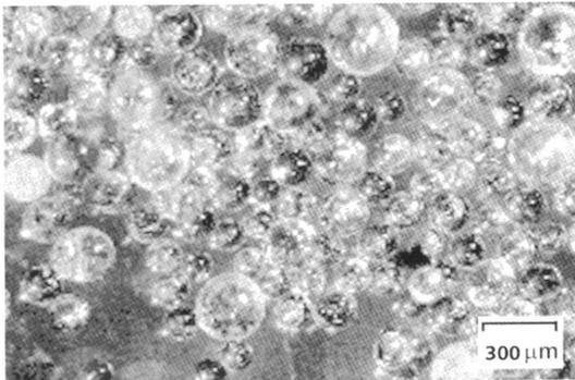
*Figure 14. Appearance of the product obtained with a single granule passage through the reactor.*
