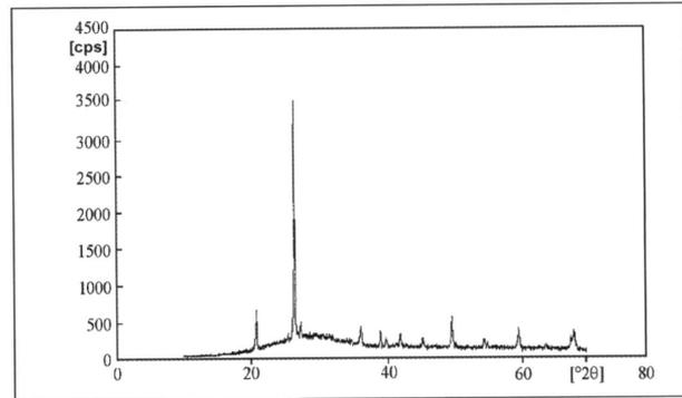
Figure 7. Diffractogram of the granules treated in the laboratory reactor at 1700°C.
