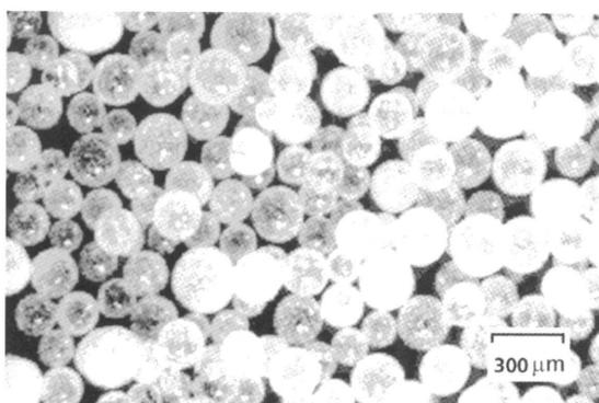
Figure 10. Granules sized <300 $\mu\text{m}$  made up of raw materials particles sized <10 $\mu\text{m}$  (90%), treated in the laboratory reactor with a lengthened chamber at 1700°C.
