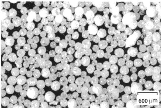
Figure 4. Granules treated in the laboratory reactor at 1500°C.
