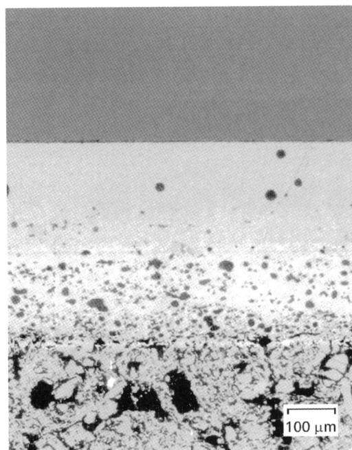
Figure 19. End glaze on applying the spheroidised frit.
