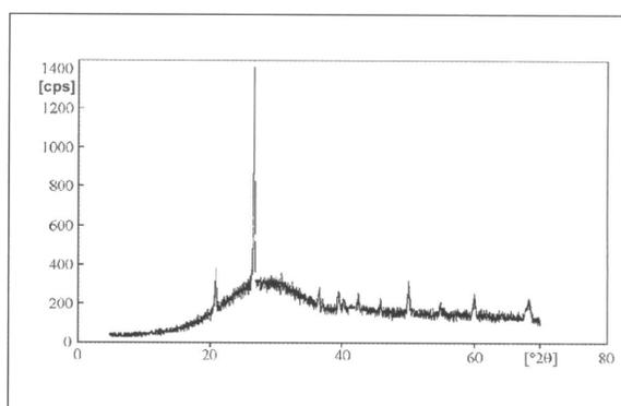
Figure 11. Diffractogram of the granules treated in the laboratory reactor at 1700°C.
