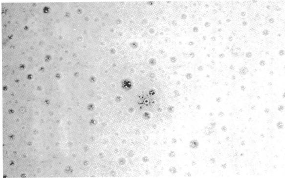
*Figure 12. Appearance of the glaze obtained with the spheroidised frit of Figures 10 and 11.*
