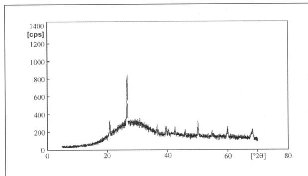
*Figure 15. Diffractogram of the product obtained with a single granule passage through the reactor.*
