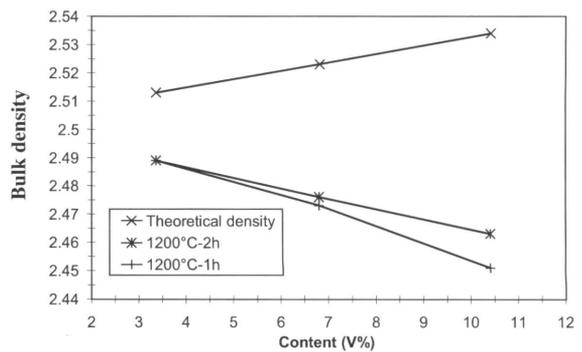
Figure 8. Bulk density as a function of the sintered mullite content for the 106-110  $\mu$ m grain size range (a same variation was observed for andalusite and  $\beta$ -spodumene)
