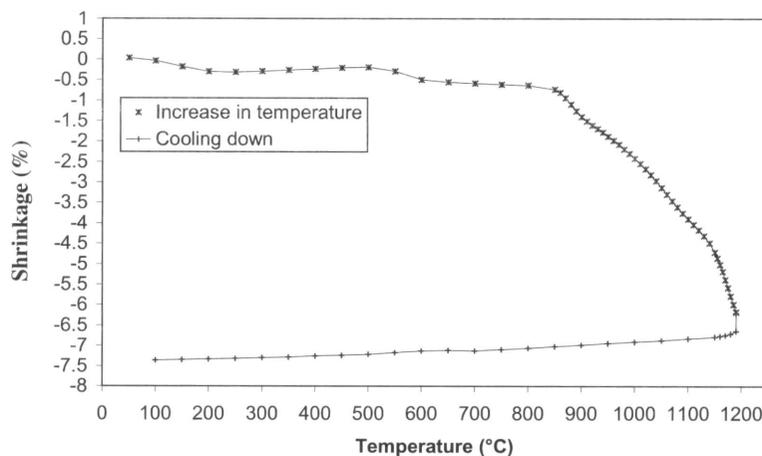
Figure 3. Dilatometric curve of an Al<sub>2</sub>O<sub>3</sub> rich composition (ratio Al<sub>2</sub>O<sub>3</sub>/SiO<sub>2</sub> ≈ 0.41) favourable to celsian crystallization.
