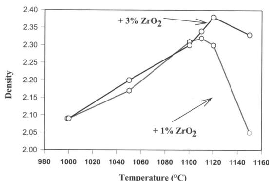
Figure 1. Effect of  $ZrO_2$  content on densification ability of the  $Li_2O$  containing composition reported in table 1
