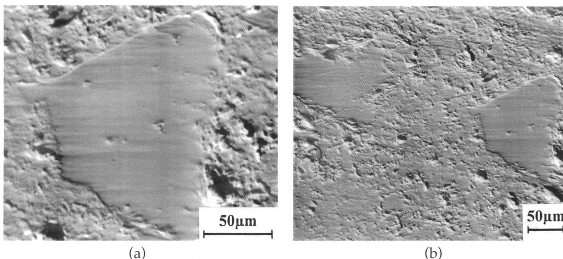
Figure 10. Agglomerate inside a sample containing andalusite : (a) BES micrograph - (b) corresponding EDX image (Al)
