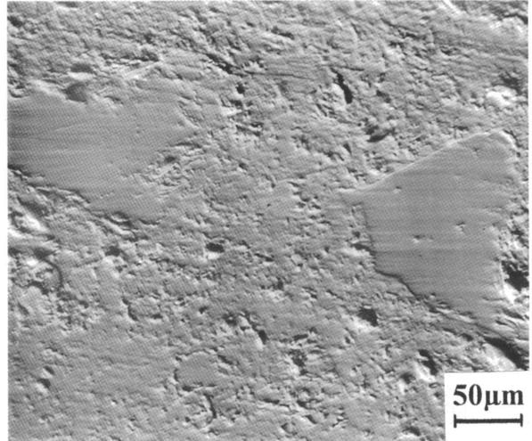
Figure 6. BSE micrograph showing no microcrack or density gradient around continuous  $\alpha$ -Al<sub>2</sub>O<sub>3</sub> grains
