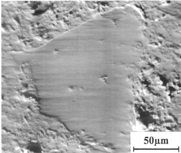
Figure 5. BSE micrograph of a single  $\alpha$ -Al<sub>2</sub>O<sub>3</sub> grain.
