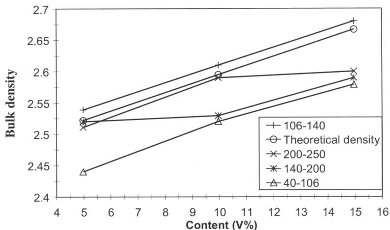
Figure 4. Bulk density as a function of the  $\alpha$ - $\text{Al}_2\text{O}_3$  content for various grain size ranges
