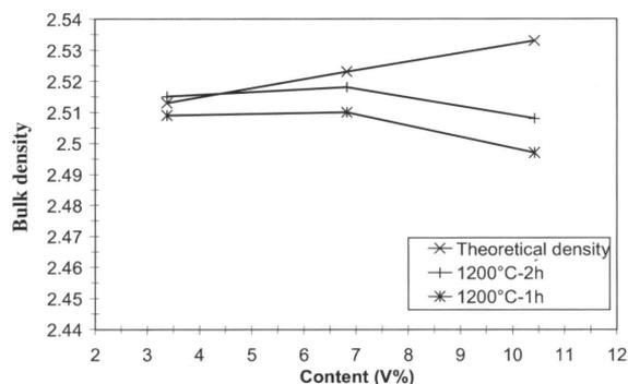
Figure 11. Bulk density as a function of the fused mullite content for the 106-110 μm grain size range.
