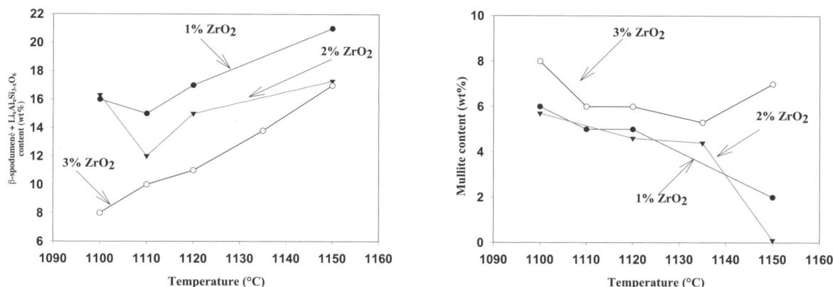
Figure 2. Effect of  $ZrO_2$  addition on crystallization of (a) Li aluminosilicate phases - (b) mullite (composition reported in table 1)
