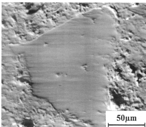
Figure 9. BSE micrograph of the microstructure of a sample containing andalusite as additional phase.
