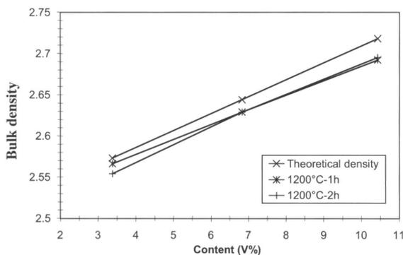
Figure 7. Bulk density as a function of the zircon content for the 106-140  $\mu$ m grain size range
