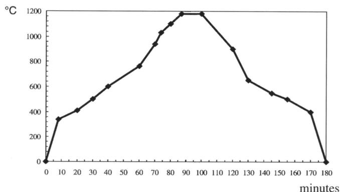
Figure 8. Firing curve for ceramic slabs.
