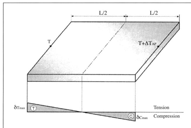
*Figure 6. Stress between the front and the rear of the piece owing to the difference in temperature.*
