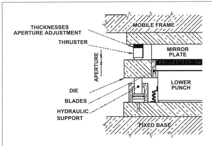
Figure 5. Schematic illustration of a mirror die with thrusters.
