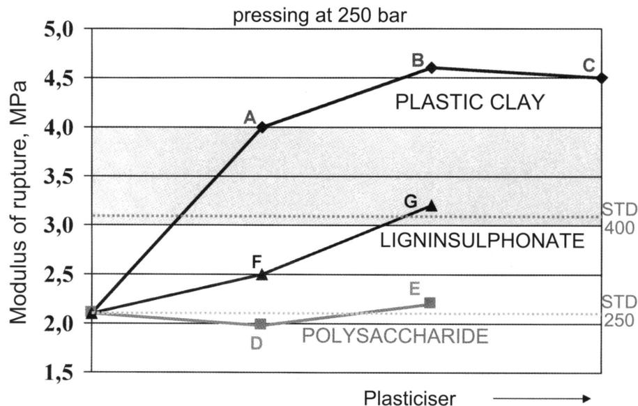
Figure 3. Effect of plasticising additives on dry mechanical strenght.
