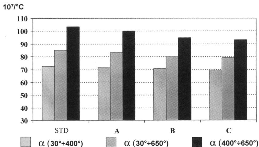
Figure 9. Linear thermal expansion of the formulated bodies.
