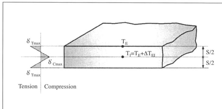
Figure 7. Stress condition owing to the difference of temperature in the thickness.
