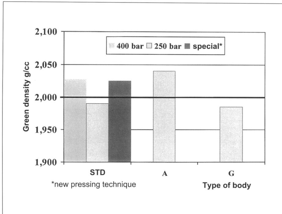
Figure 4. Variation of compaction density according to type of body and pressing.
