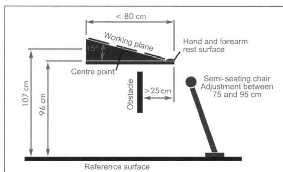
Figure 13. Recommended workstation design for discontinuous tile feed or carpet of tiles.
