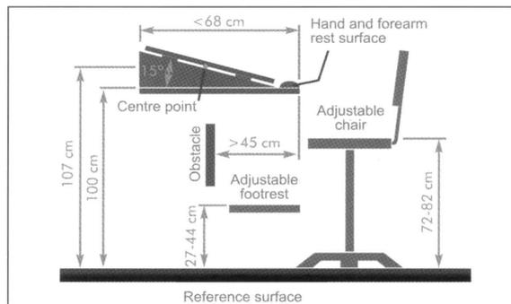
Figure 15. Recommended workstation design for continuous tile feed with selection by fluorescent fibre-tip pen.
