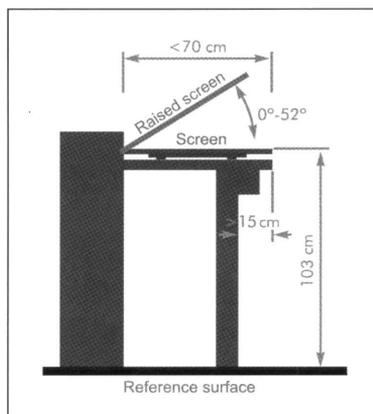
Figure 19. Recommended screen printing workstation design with a front-opening screen.
