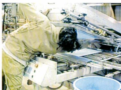
Figure 12. Printing screen with an excessive front reach imposed by the control panel.
