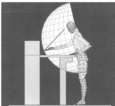
Figure 20. Recommended screen printing workstation design with a front-opening screen..
