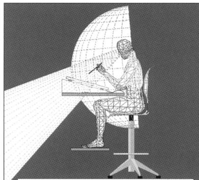
Figure 16. Recommended workstation design for continuous tile feed with selection by fluorescent fibre-tip pen.
