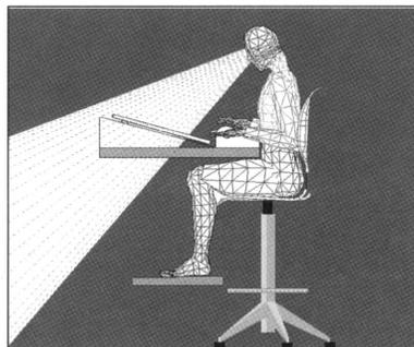
Figure 18. Recommended workstation design for continuous tile feed with selection by mouse or mobile keyboard.
