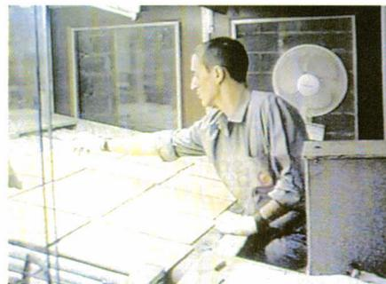
*Figure 7. Elements of the bench that hinder reaching the tiles.*
