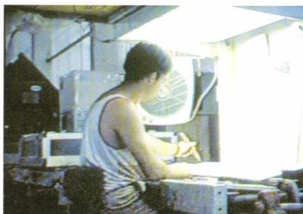
*Figure 4. Continuous tile feed, with selection by a fluorescent fibre-tip pen.*
