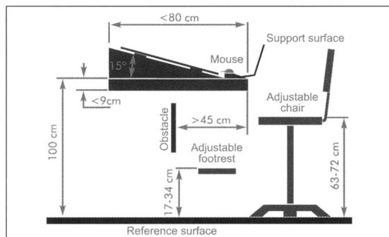
Figure 17. Recommended workstation design for continuous tile feed with selection by mouse or mobile keyboard.
