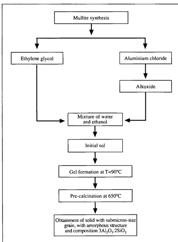
Figure 3. Schematic illustration of the mullite gel processing stages by the polymer sol-gel method.
