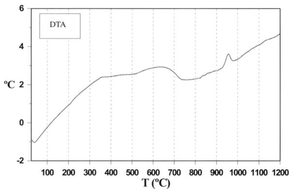
*Figure 11. DTA curve of the frit B-corundum gel hybrid material, showing the  $T_g$  region and crystallisation exothermic peak.*
