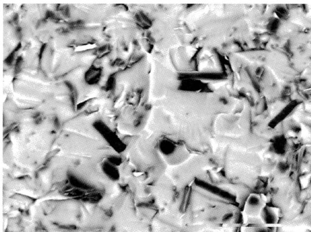
*Figure 13. SEM image obtained using a back-scattered electron detector showing dark-coloured corundum crystals with tabular and fibrous shapes and a crystal-size distribution ranging from 1 to 3 μm.*
