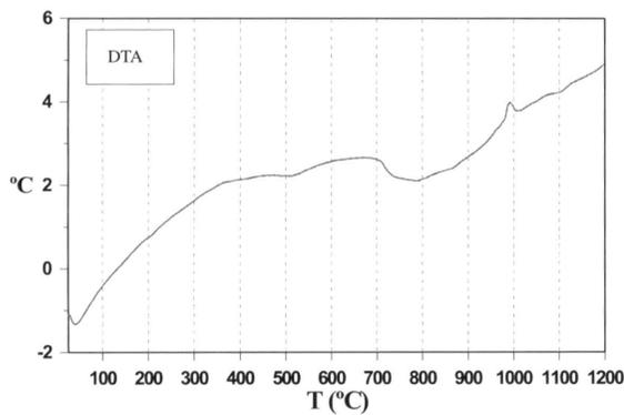
Figure 8 DTA curve of the frit A-mullite gel hybrid material, showing the  $T_g$  region and crystallisation exothermic peak.
