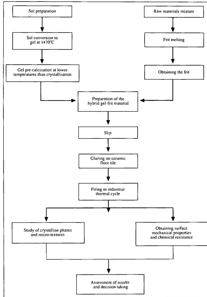
Figure 1. Logical flow chart of the various work stages for achieving the main objectives and producing glass-ceramic glazes with advanced properties compared to conventional glazes.
