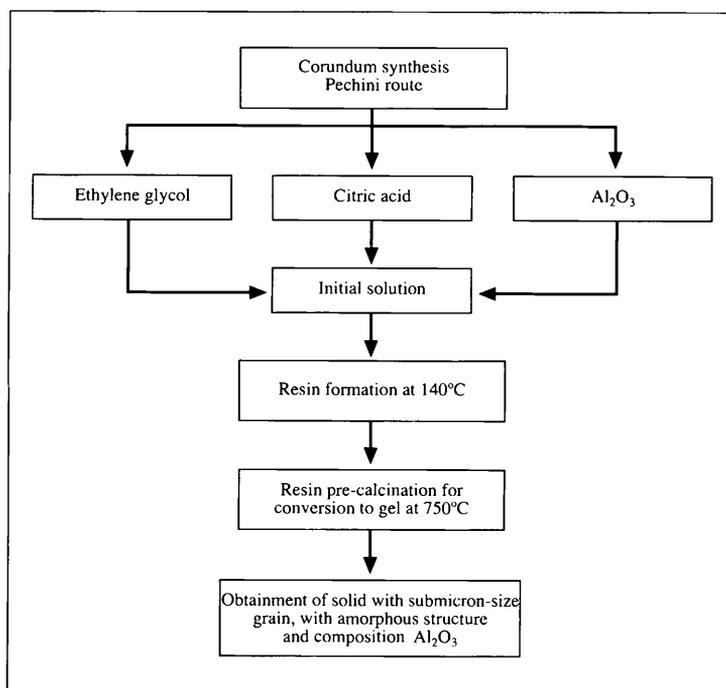
Figure 2. Schematic illustration of corundum gel processing by the Pechini method.
