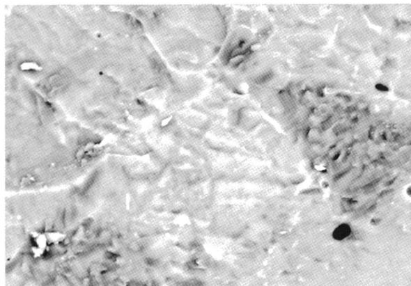
Figure 10. SEM image obtained using a back-scattered electron detector, showing oval regions with a darker colour, which correspond to mullite and corundum crystallisation, and a centre region exhibiting tabular anorthite crystals.
