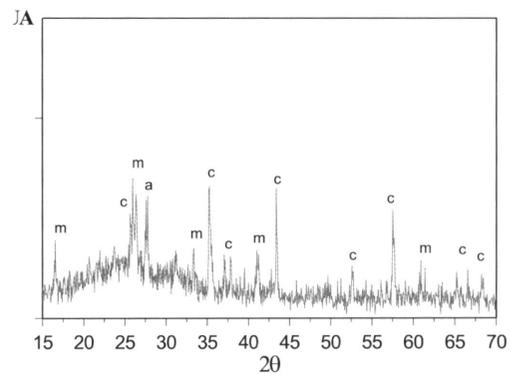
Figure 9. Diffractogram of the specimen glazed and fired with the hybrid material, showing the mullite phase (m), together with corundum (c) and a very minor anorthite (a) phase.
