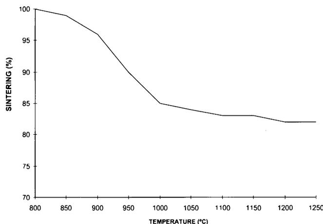
Figure 15. Sintering curve of the mullite glass-ceramic material, plotting sintering percentage versus temperature.
