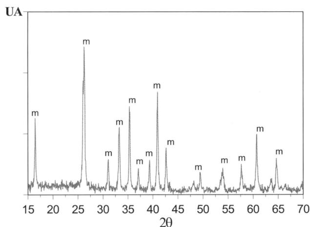
Figure 5. Diffractogram of the mullite gel heated according to the porcelain tile industrial cycle (1200°C/15 min), developing the mullite of crystalline phase as sole species.
