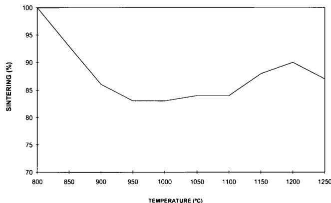
Figure 14. Sintering curve of the corundum glass-ceramic material, plotting sintering percentage versus temperature.
