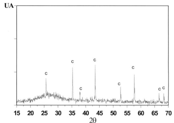
*Figure 12. Diffractogram of the specimen glazed and fired with the hybrid material, showing the corundum phase to be the sole crystallising species.*
