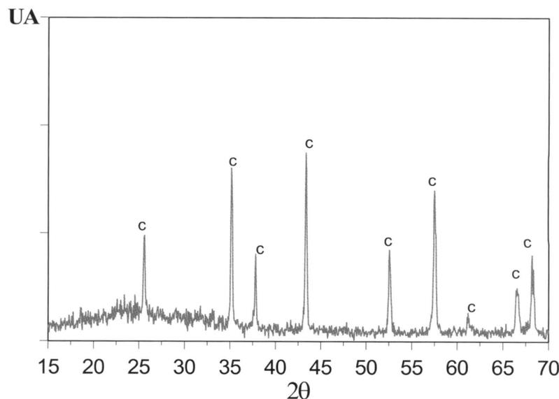
Figure 7. Diffractogram of the corundum gel heated according to the porcelain tile industrial cycle (1200°C/15 min) developing a corundum crystalline phase as sole species.
