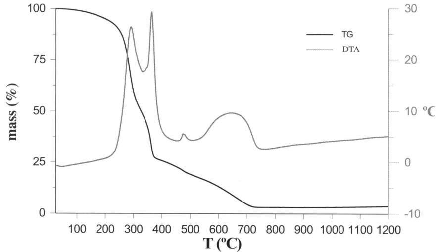
Figure 6. DTA and TG curves of the Pechini resin for corundum synthesis, presenting the most important transformations with temperature.
