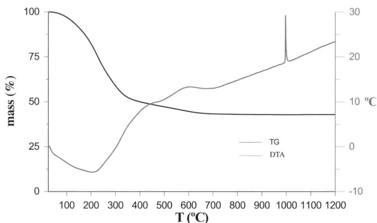
Figure 4. DTA and TG curves of the mullite gel obtained on heating at 25°C/min, showing the basic transformations with the heating process.
