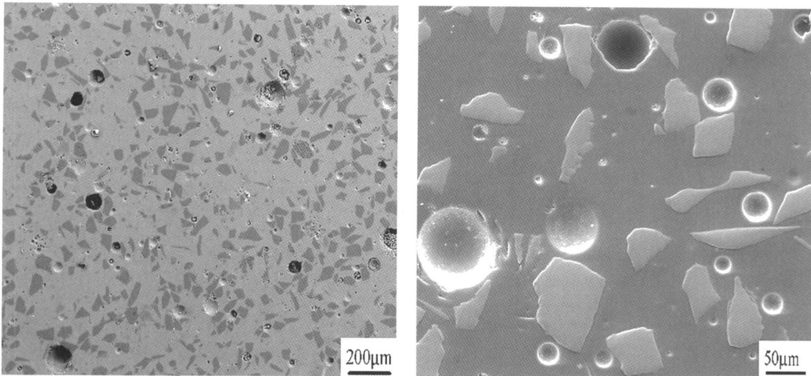
Figure 1. Composites containing: (a) 20 vol% mullite and (b) 25 vol% zirconia.
