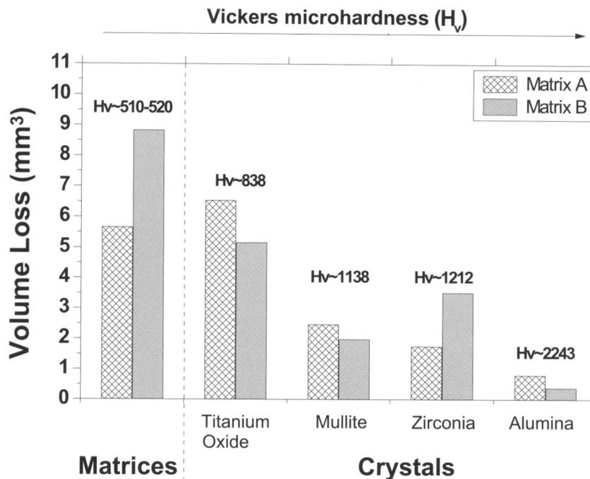
Figure 4. Correlation between material volume loss (in specimens with 10% crystals, after a 10-min wear test) and Vickers microhardness of the matrices and crystals separately.
