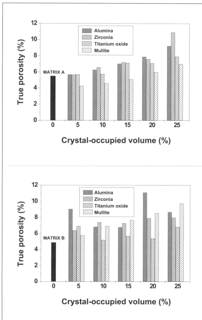
Figure 2. True porosity for composites with different crystal addition contents in matrices A and B.
