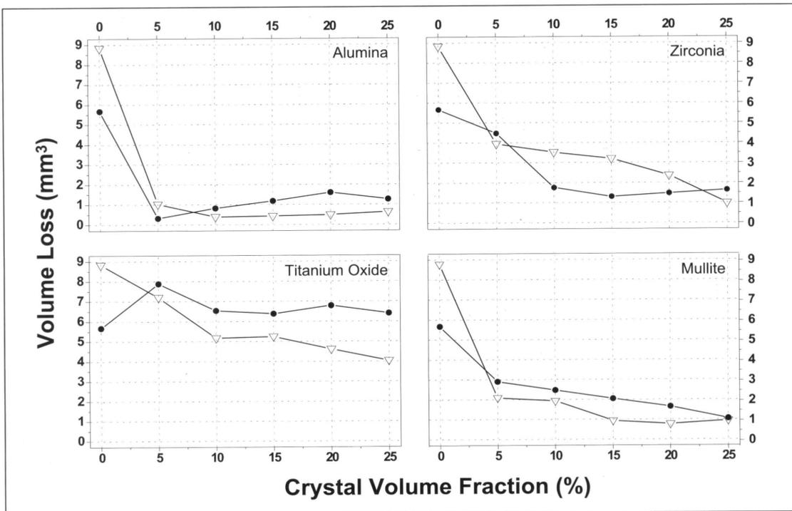
Figure 3 . Volume loss found for matrix A (—●—) and B (—▽—) composites, after a 10min wear test.
