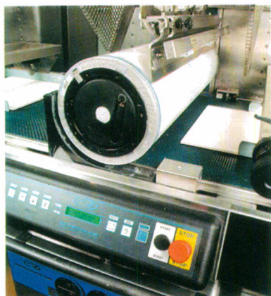
Figure 21. Printing roll of a rotogravure decorating machine.
