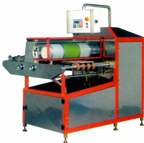
Figure 25. Flexography decorating system.
