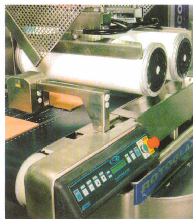
Figure 12. Rotogravure glazing system.
