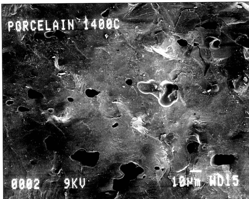
*Figure 4. SEM Micrograph of a porcelain body fired at 1400°C showing a high degree of vitrification.*
