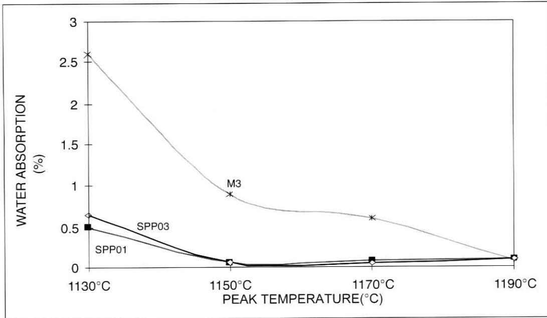
Graph 1. Vitrification Curve Of Vitrified Tile Bodies With Water Absorption Vs Firing Temp.
