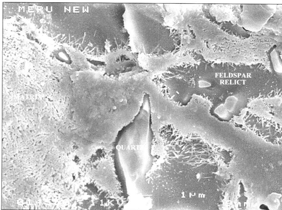
*Figure 2. SEM Micrograph of the typical features of a vitrified body showing the quartz grain with its solution run, the pools of glass representing feldspar relicts and the dense matrix, mostly mullite (brighter areas) with some glass (darker areas)*
