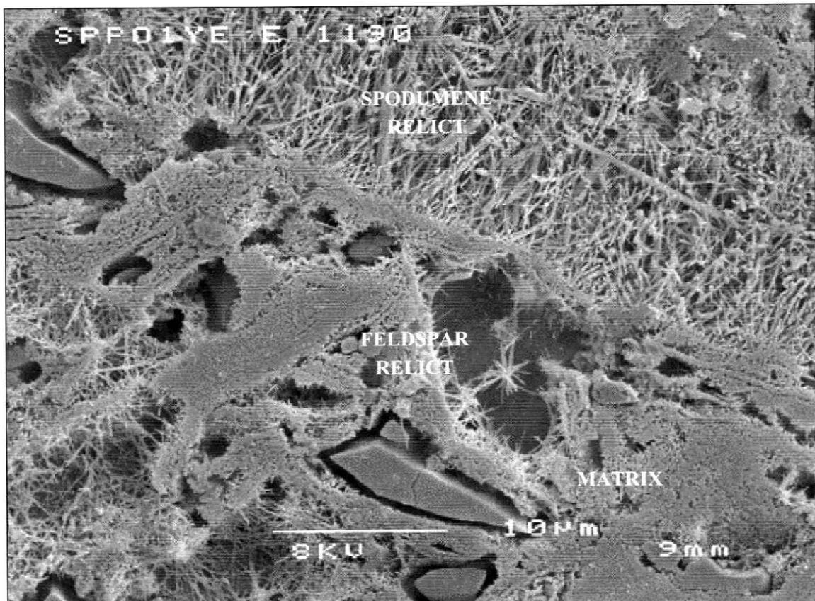
Figure 1. SEM Micrograph of a vitrified body with spodumene showing a greater density of mullite crystals in the spodumene relict compared with the feldspar one.
