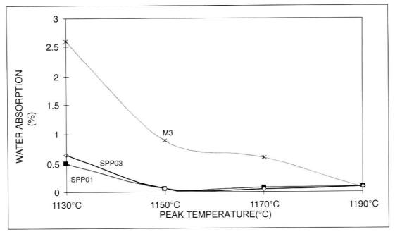
Graph 1. Vitrification Curve Of Vitrified Tile Bodies With Water Absorption Vs Firing Temp.
