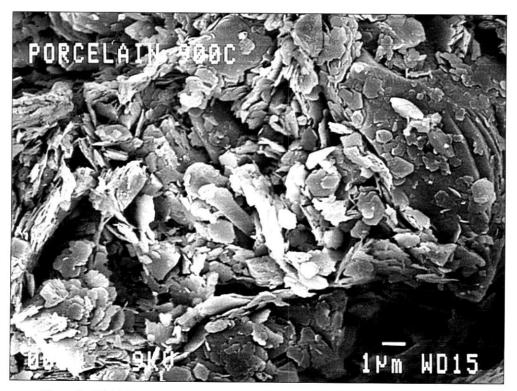
Figure 3. SEM Micrograph of a porcelain body fired at 900°C showing very little melting.
