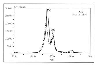
Figure 1. Zirconium silicate peak in specimens A-C and A-1140.
