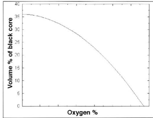
*Figure 2. Evolution of the elimination of black core as a function of atmosphere for the trial composition.*
