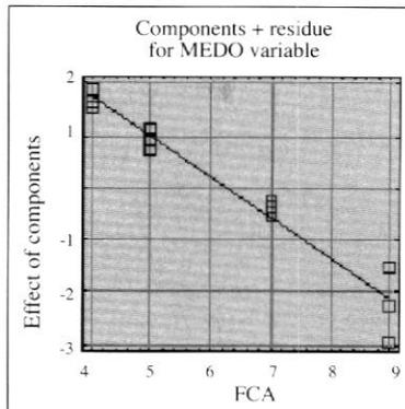
Figure 7. Regression model between variation of ink viscosity and off-contact. Analysis was performed at a constant screen tension of 20 N/cm.
