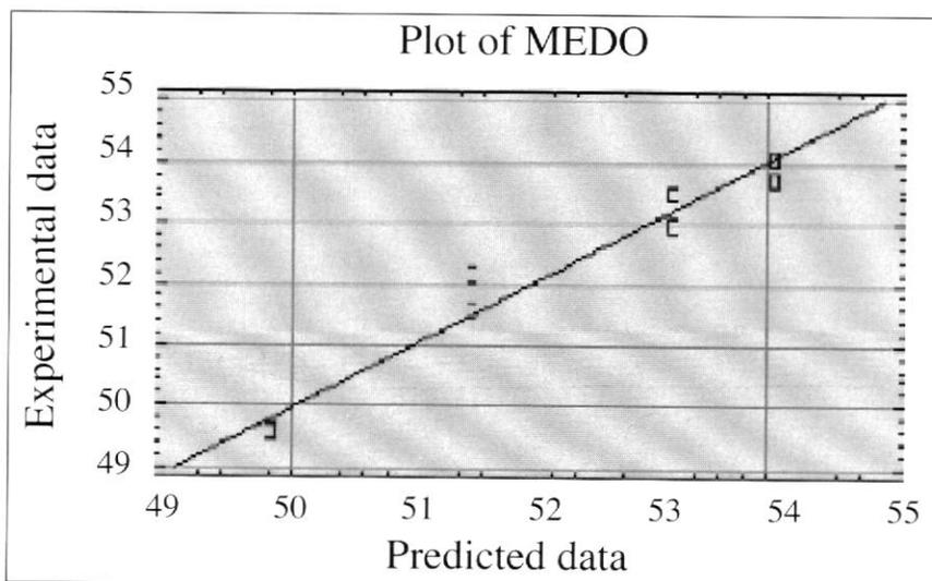
*Figure 4. Plot of MEDO for experimental and predicted values using the model, corresponding to Table 2, between the mean L value for the grey reference value found for each specimen and “off-contact” in mm. The data were obtained at a constant viscosity and screen tension. On raising “off-contact”, L dropped and the specimen became a darker shade.*
