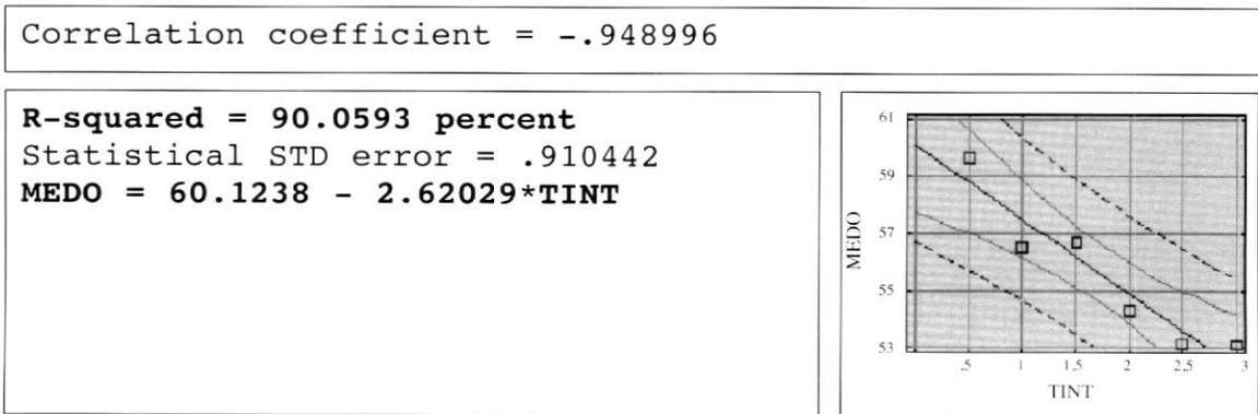
*Figure 9. Analysis of linear correlation between viscosity and variation in printed colour. Raising viscosity produced a darker image.*
