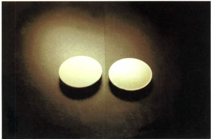
Figure 6. Appearance of fired specimen fair faces: a) Non-treated specimen; b) Treated specimen with immediate drying
