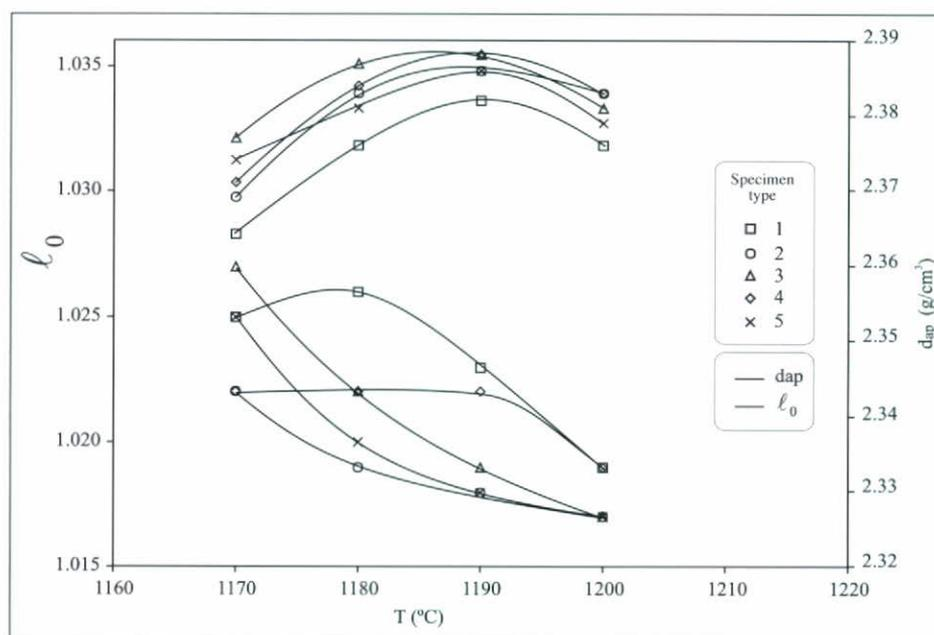
Figure 4. Variation of ℓ<sub>0</sub> and d<sub>ap</sub> of the fired specimens with firing cycle T<sub>max</sub>.
