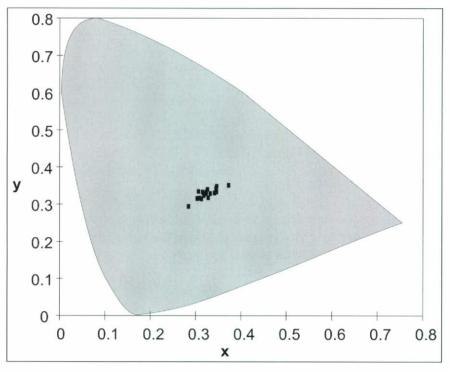
Figure 3. Situation of the tested ink coordinates in the colour space.
