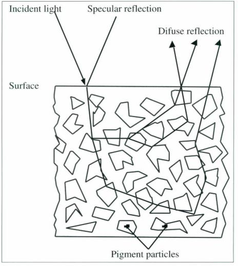
Figure 2. Interaction of light with pigmented objects.
