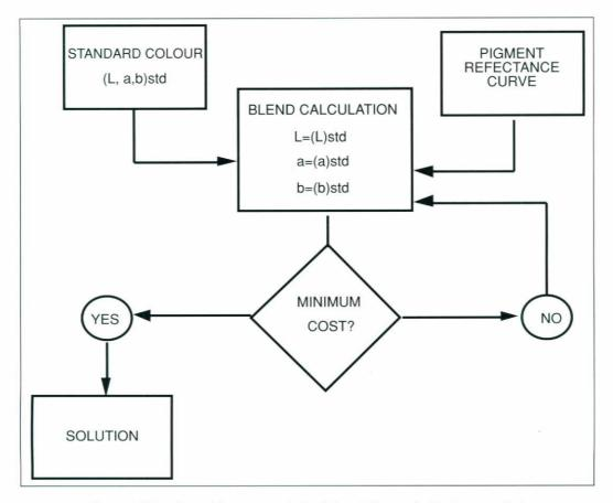
Figure 4. Flow chart of the screen-printing ink matching and adjustment method.
