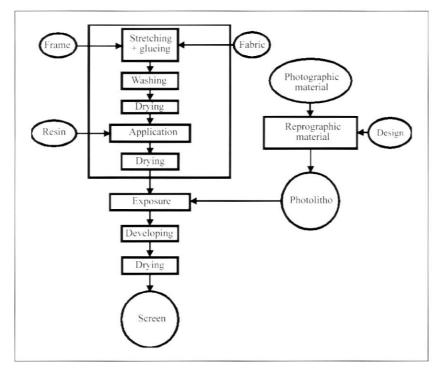
Figure 1. Schematic of the printing screen production process.
