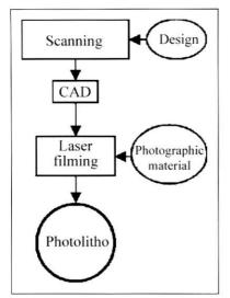
Figure 4. Schematic of photolitho preparation by filming.
