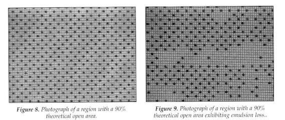
Table 4 indicates the characterisation results of the 18 screens corresponding to experiment design. For brevity only the percentage increase in open area (emulsion loss) produced in developing is given in the table, together with weight loss and decreased thickness found in the different screens on undergoing 1000 abrasion cycles.
