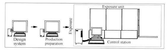
Figure 7. Screen production by the DISE 3 system
