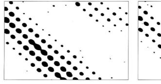
*Figure 2.Photograph of a given area* of an original photolitho (magnification 19x)
