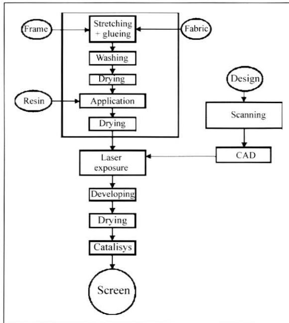
Figure 5. Schematic of the printing screen preparation process by laser exposure.
