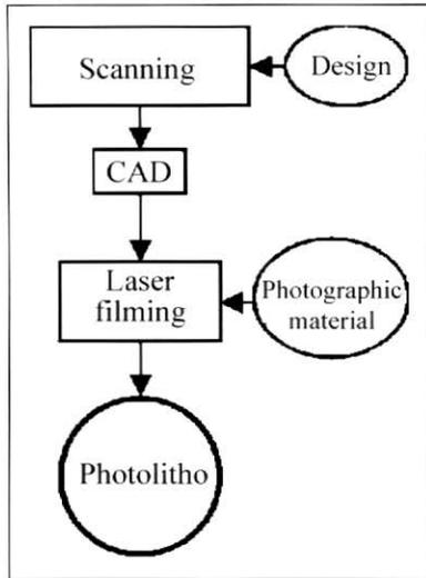
Figure 4. Schematic of photolitho preparation by filming.
