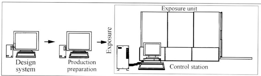
Figure 7. Screen production by the DISE 3 system
