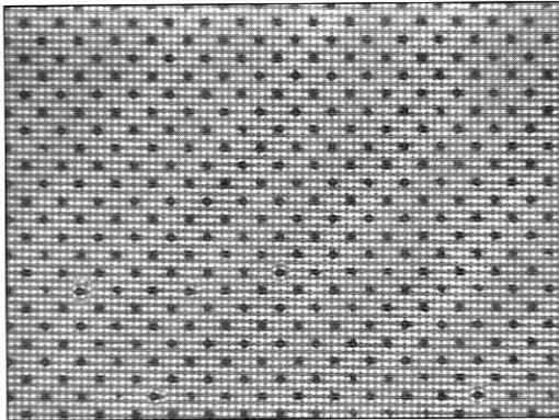
Figure 8. Photograph of a region with a 90% theoretical open area.
