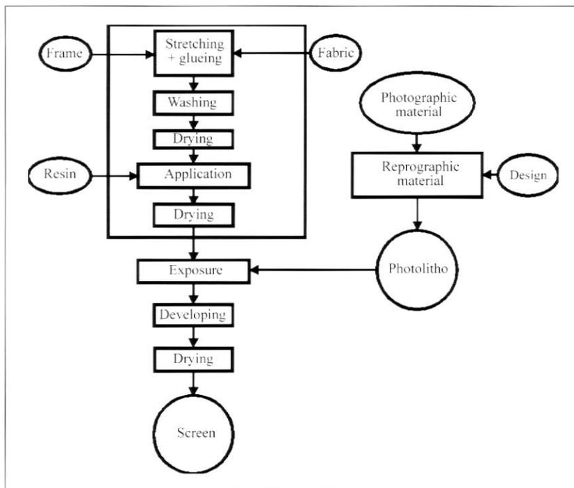
Figure 1. Schematic of the printing screen production process.
