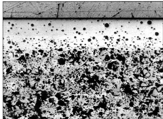
Figure 15. Polished cross section of glaze IB.
