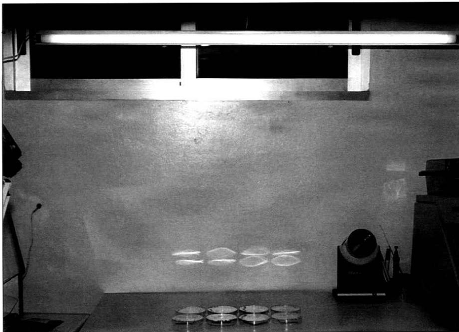
*Figure 11. Experimental assembly used for lighting the petri dishes containing the ceramic specimens sown with the selected bacteria.*
