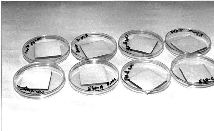
*Figure 10. Glazed ceramic specimen distribution. Trials were run with the conventional glaze (control trials) and with the bactericidal glaze.*
