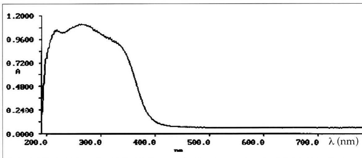
Figure 7. Bactericidal glaze absorption spectrum.
