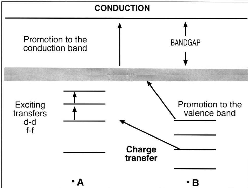
Figure 1. Electron transfers in solids affecting optical properties. Energy levels are shown for two atoms, A and B, together with some characteristic electronic states in solids.
