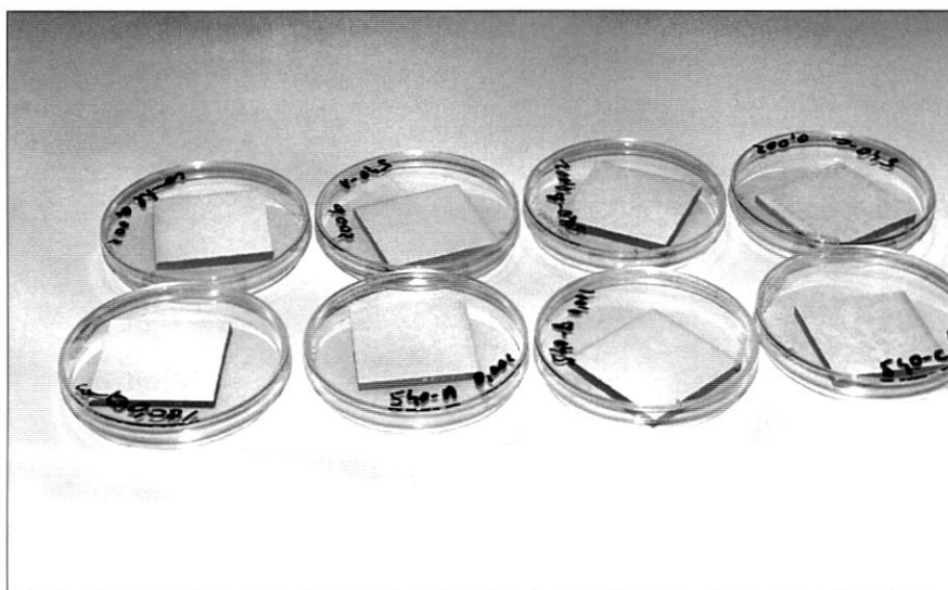
Figure 10. Glazed ceramic specimen distribution. Trials were run with the conventional glaze (control trials) and with the bactericidal glaze.
