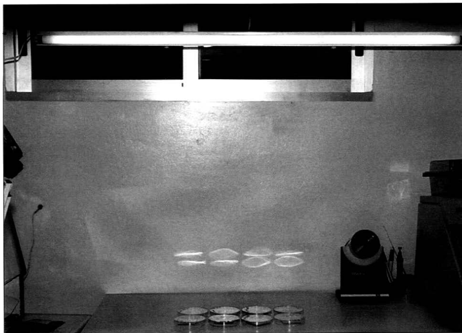
Figure 11. Experimental assembly used for lighting the petri dishes containing the ceramic specimens sown with the selected bacteria.
