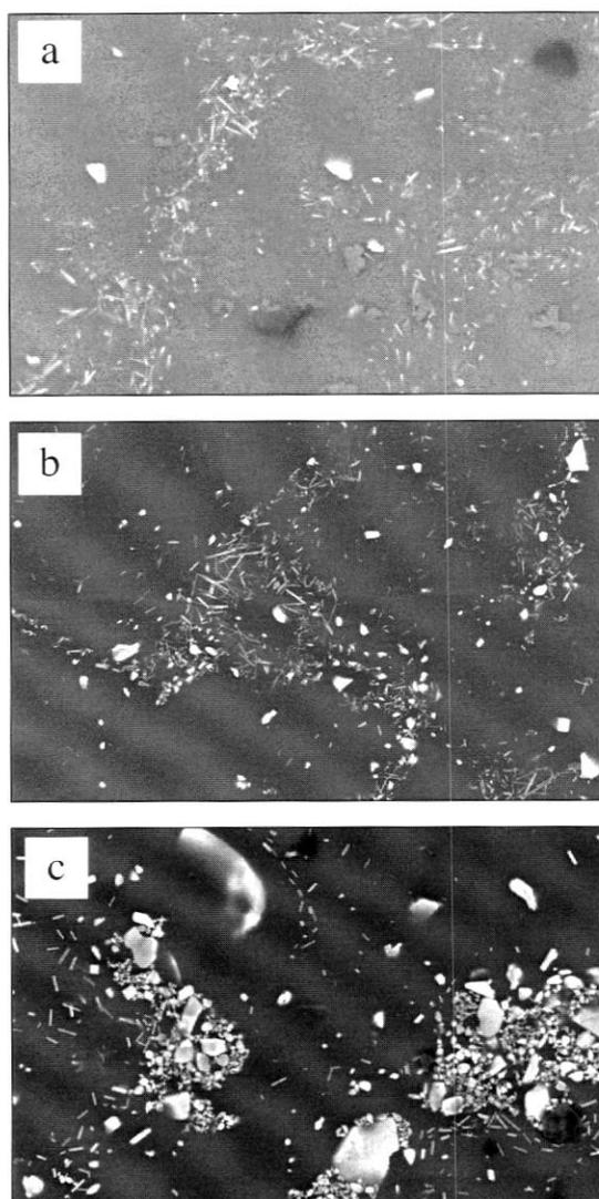
Figure 3. SEM micrographs with back-scattering detector of the cryolite  $Na_3AlF_6$  additions to base A: (a)1%,(b)3%,(c)10%.
