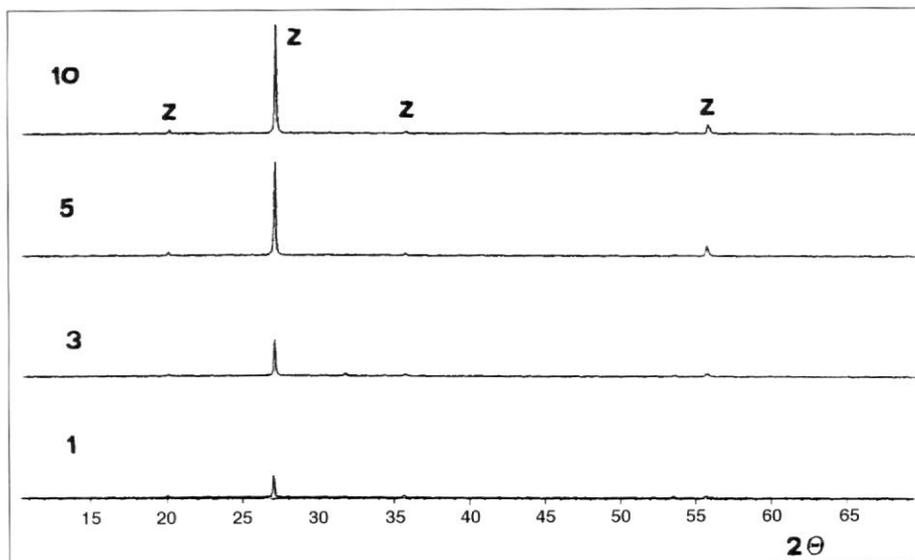
Figure 2. XRD of the cryolite  $Na_3AlF_6$  additions to base A: (a)1%,(b)3%,(c)5%,(d)10%.
