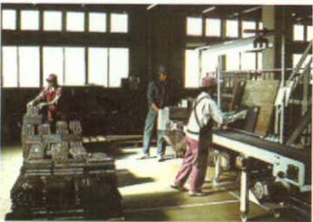
*LEFT. Manufacturing process of the ceramic material used in the outside veneer of the Nara Convention Hall.*
