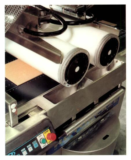
The concept of parallel glazing and decoration is loaded with meanings and possibilities, in as much as it allows eliminating a constraint on decoration: parallel-glazed tiles with ROTOGLAZE can be parallel-decorated by ROTOCOLOR on receiving different portions of a decoration that can lie across the whole decorating roller surface.
