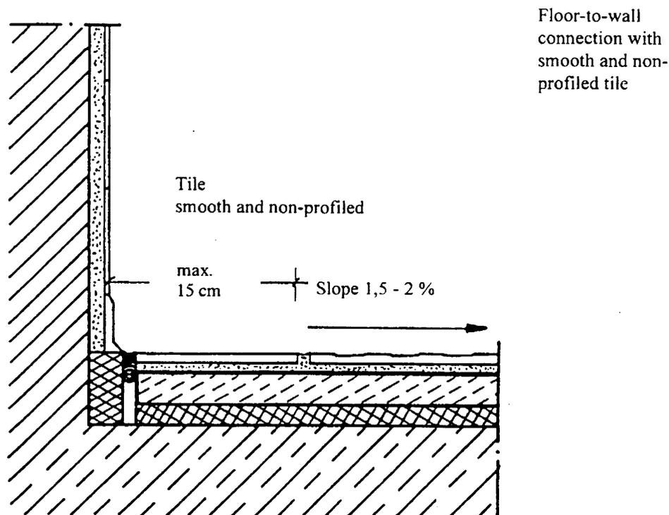
If mosaics are laid in wet areas, only mosaics with papering on the face sides must be used in order to obtain optimum adhesion and fully saturated laying. Mosaics with paper-net on the reverse sides normally only provide an adhesion surface of approximately 63 - 75 percent. For this reason, a fully saturated coating of the tile reverse side as required by DIN 18157, part 1, section 7.3.3, is impossible even if applying the combined laying method.
