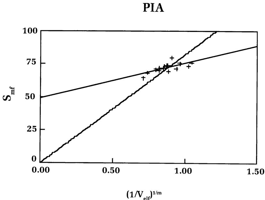
**Figure 2:**  $S_{\text{mf}}$  versus  $(1/V_{\text{eff}})^{1/m}$  for the PIA fracture model. The solid line is according to equation (3), the dashed line is according to the anomalous statistical model by Scholten et al. [7] (equation (4)).
