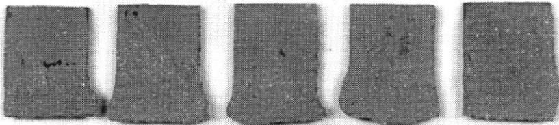
TILE: POROUS (RED BODY) - ADHESIVE: TYPE A (CEMENTITIOUS ADHESIVE) - TEST: SHEAR
