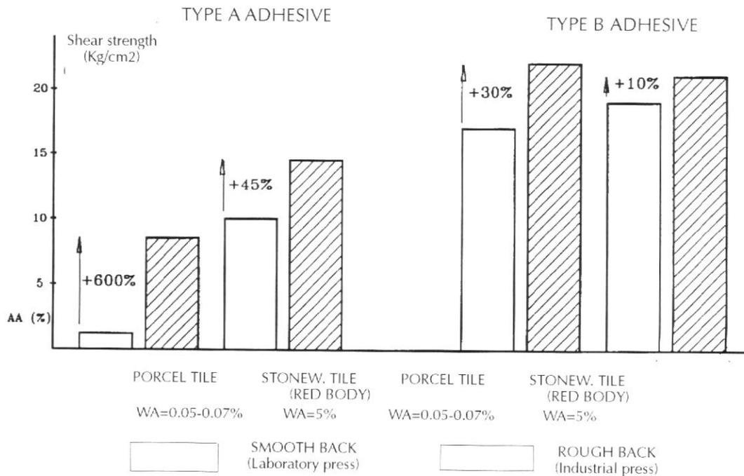
been observed that adhesive applications of this thickness lead to faulty installation (with a large number of cavities and small cracks in the setting). These facts counsel against the use of «aggressive» ribs with these adhesives, installed with the thin-set method, especially if we take into account the difficulty involved in achieving the proper application of adhesive on the back of a tile with excessive relief.
