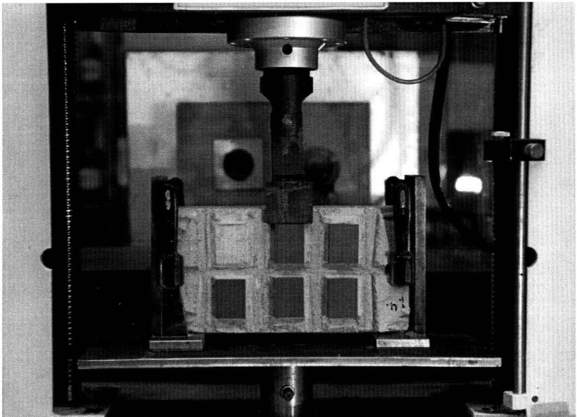
PHOTOGRAPH 2: DETAIL OF DEBONDING BY SHEAR LOADING
