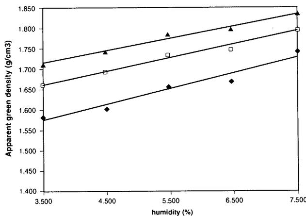
Figure 2 - Apparent green density (d) plotted against humidity content (h) for three pressures of compaction (◆ p<sub>1</sub> = 22 MPa, ■ p<sub>2</sub> = 45 MPa, ▲ p<sub>3</sub> = 67 MPa). Correlation factors (r): r<sub>1</sub> = 0.97, r<sub>2</sub> = 0.99, r<sub>3</sub> = 0.99.
