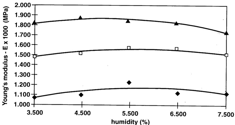
Figure 4 - Young's modulus (E) plotted against humidity content (h) for three pressures of compactation (◆ p<sub>1</sub> = 22 MPa, ◻ p<sub>2</sub> = 45 MPa, ▲ p<sub>3</sub> = 67 MPa).
