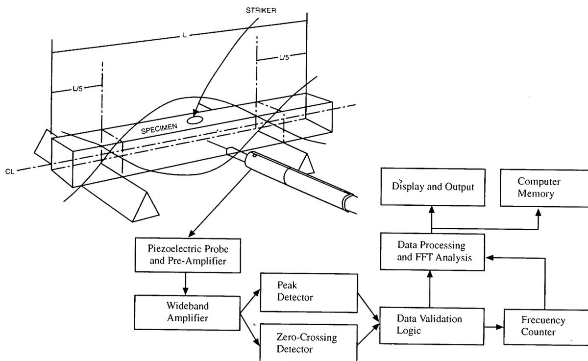
Figure 1 - Schematic diagram of the instrumentation used for the impulse excitation resonant frequency testing [3, 8].
