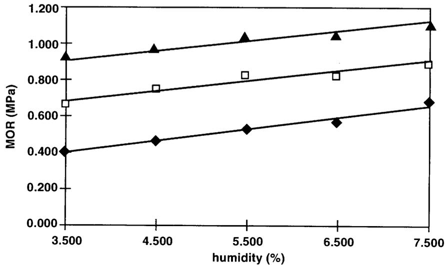
Figure 3 - Flexural strength (MOR) plotted against humidity content (h) for three pressures of compactation (◆ p<sub>1</sub> = 22 MPa, ◻ p<sub>2</sub> = 45 MPa, ▲ p<sub>3</sub> = 67 MPa). Correlation factors (r): r<sub>1</sub> = 0.98, r<sub>2</sub> = 0.96, r<sub>3</sub> = 0.96.
