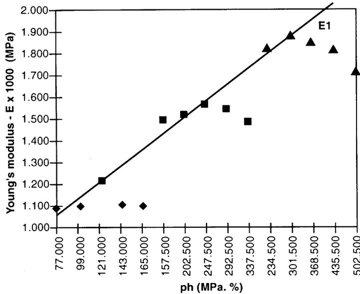
Figure 5 - Young's modulus (E) plotted against the product of the pressure of compaction (p) and humidity content (h).  $\blacklozenge$   $p_1 = 22$  MPa,  $\blacksquare$   $p_2 = 45$  MPa,  $\blacktriangle$   $p_3 = 67$  MPa) for  $3.5 \leq h \leq 7.5\%$  constant. Correlation factor (r):  $r_1 (E_1) = 0.98$ .
