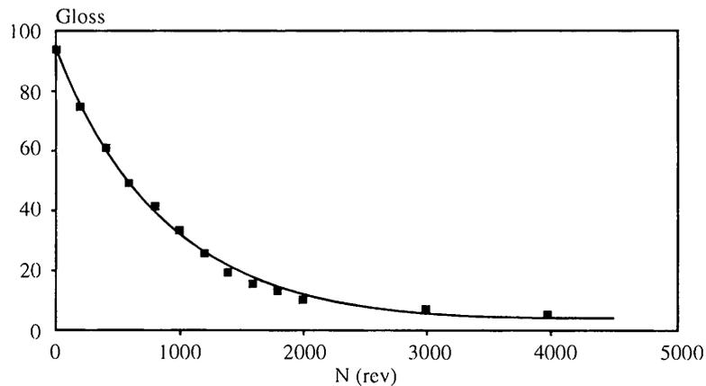
Figure 1. Evolution of glaze gloss with the number of revolutions of the abrasion tester.
