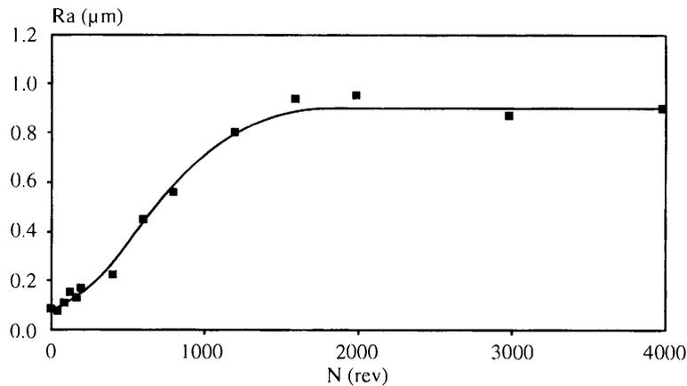
Figure 2. Evolution of parameter Ra of a glaze with the number of revolutions of the abrasion tester.
