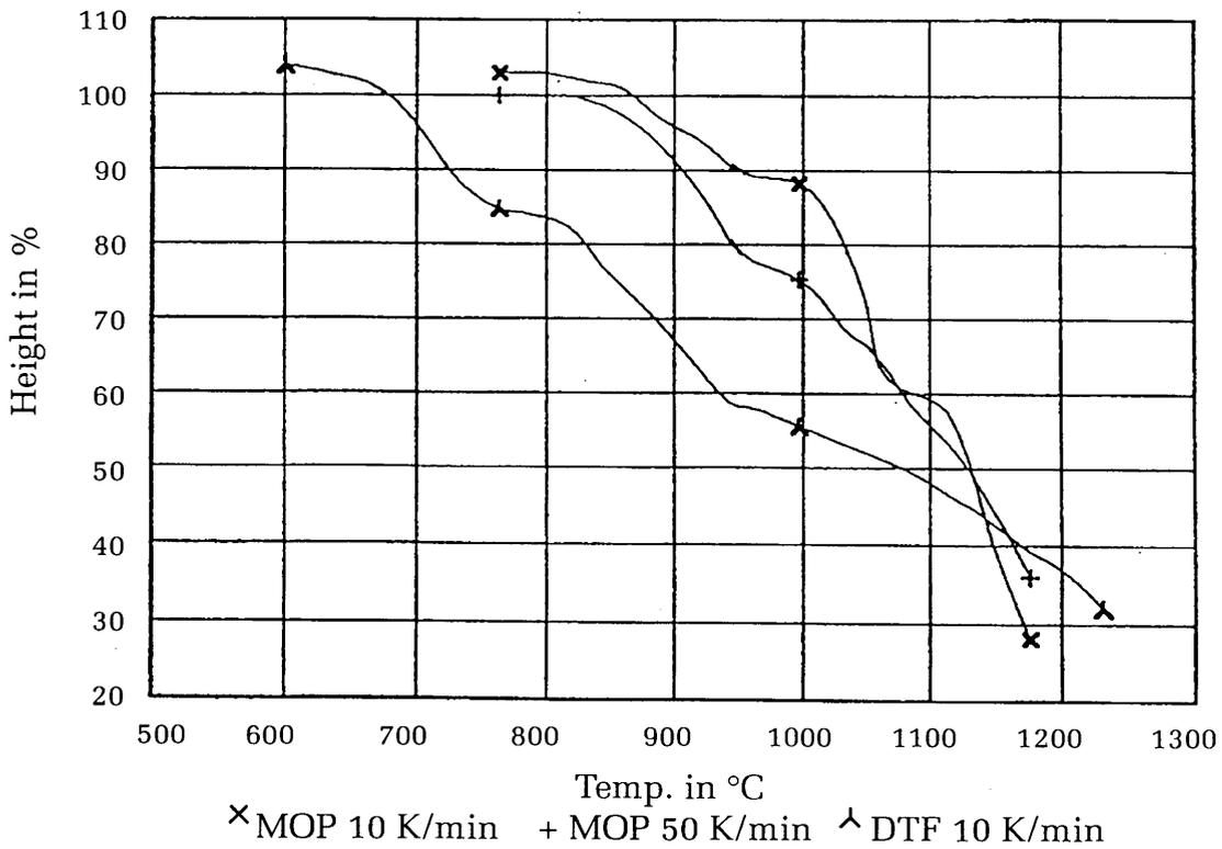
Fig. 6: Comparison between a Monoprosa and Traditional White Frit
