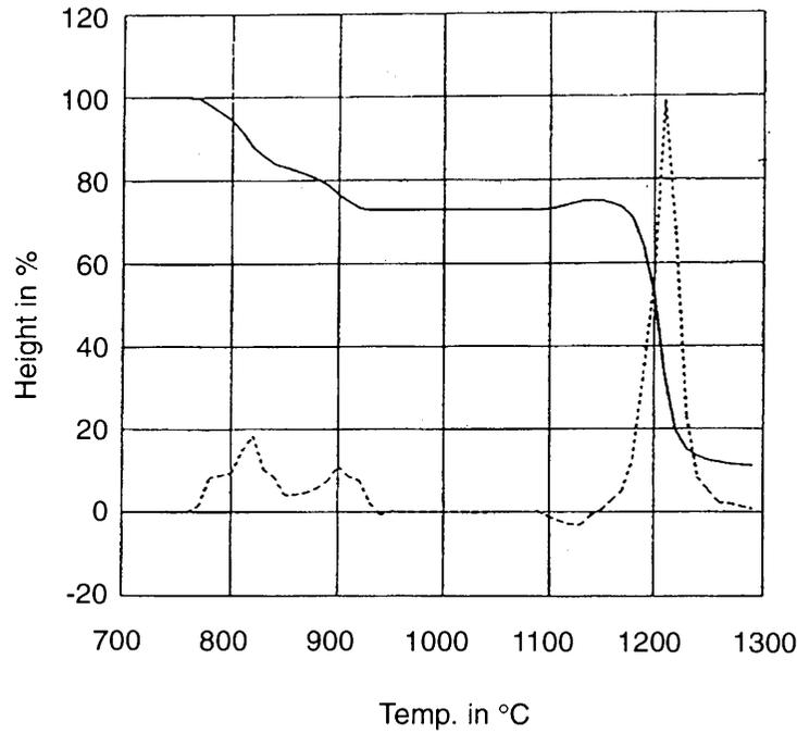
Fig. 7: Single Fast Firing Ca-Matte frit.
