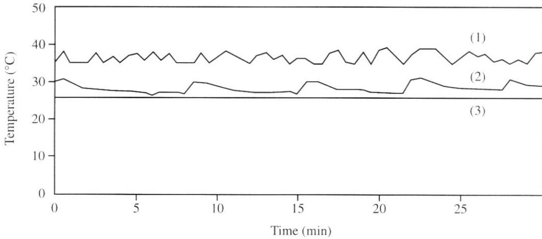
**Figure 3.** Evolution of tile (1), ink (2) and ambient (3) temperatures.
