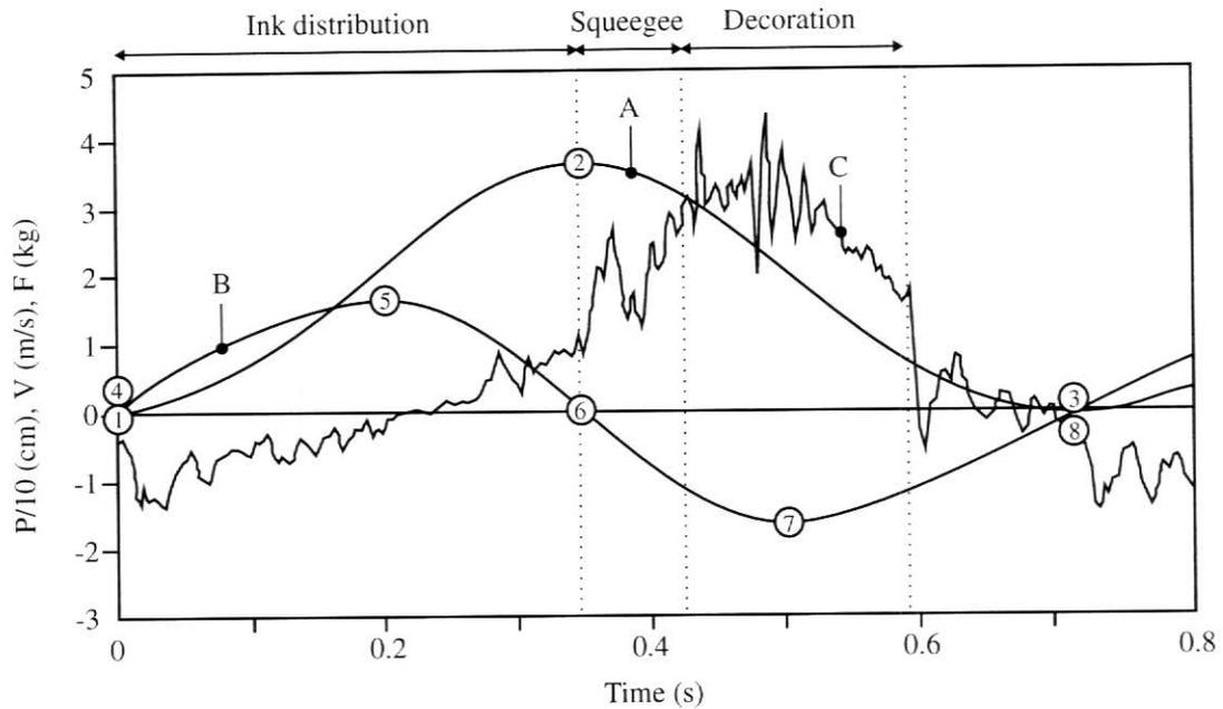
Figure 2. Evolution of the squeegee position, velocity, and force during a printing cycle.
