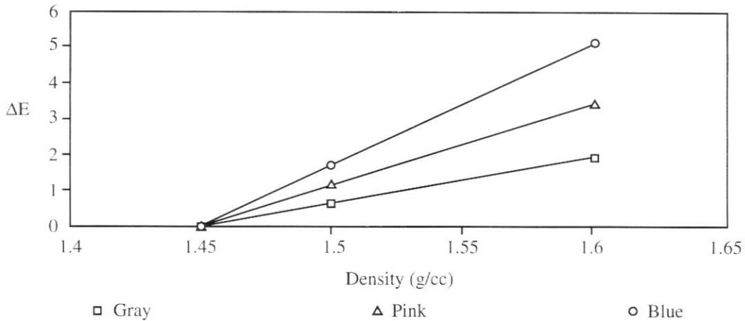
Figure 5. Influence of ink density on screen-printed colours
