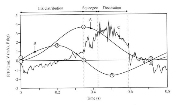
Figure 2. Evolution of the squeegee position, velocity, and force during a printing cycle.
