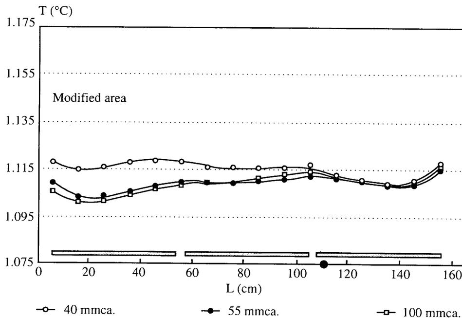
Figure 7. Transverse temperature profiles obtained on modifying burner combustion air pressure on the left side of the kiln.
