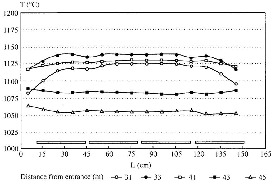
Figure 3. Transverse temperature profiles in the firing zone under the roller plane.
