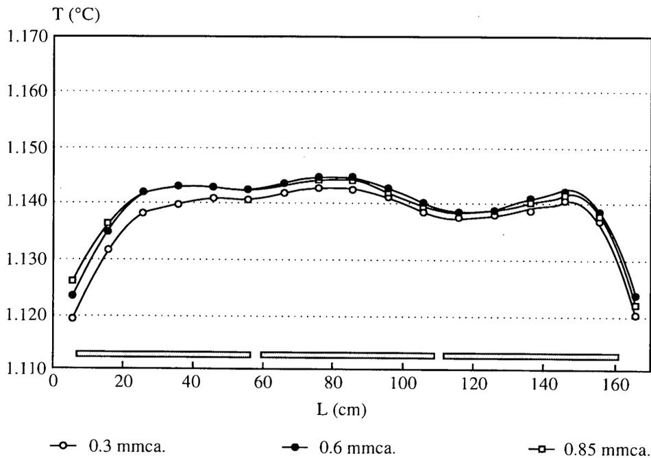
**Figure 9.** Variation of transverse temperature gradients on modifying gas static pressure in the kiln.
