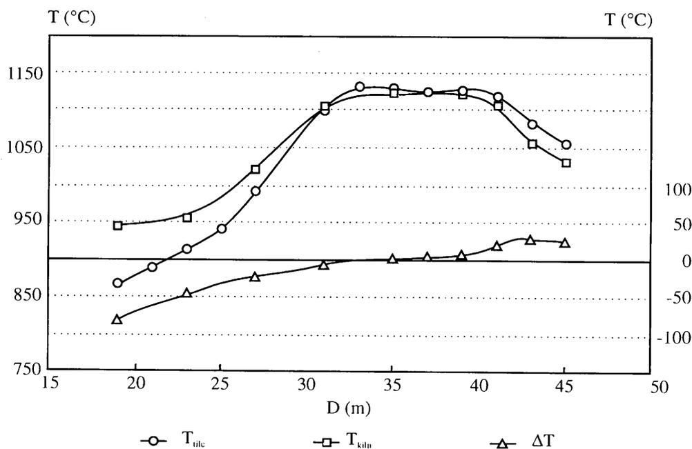
**Figure 1.** Difference between mean tile temperature and the temperature measured by the kiln thermocouples beneath the roller plane.
