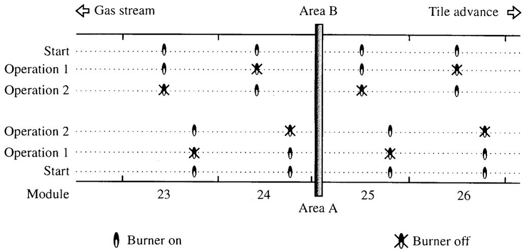
Figure 5. Detail of the tested burner arrangements beneath the roller plane
