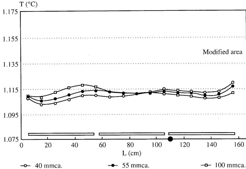
**Figure 8.** Temperature profiles obtained on modifying burner combustion air pressure on the right side of the kiln.
