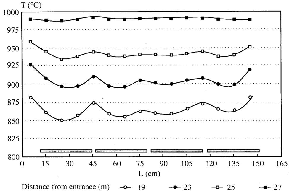
Figure 2. Transverse temperature profiles in the preheating zone under the roller plane.
