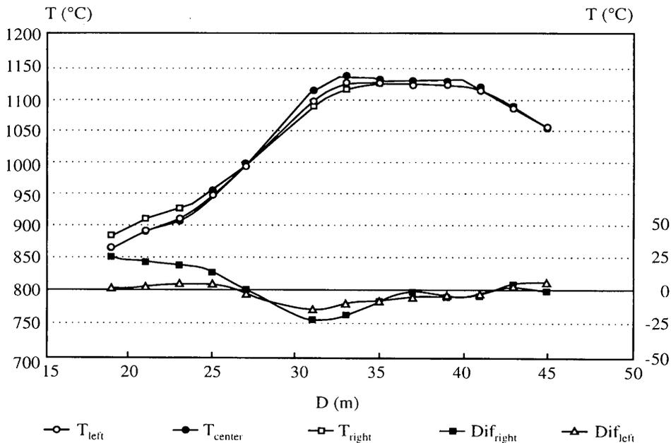
Figure 4. Heat-treatment cycles of the tile edges fired next to the kiln wall and of the tile centre fired in the middle of the kiln.
