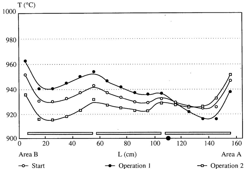
Figure 6. Transverse temperature profiles at the measuring point on modifying the number of operating burners.
