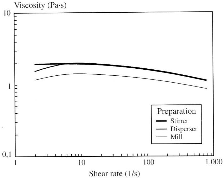
**Figure 13.** Ink L4 viscosity curve with different preparation systems.
