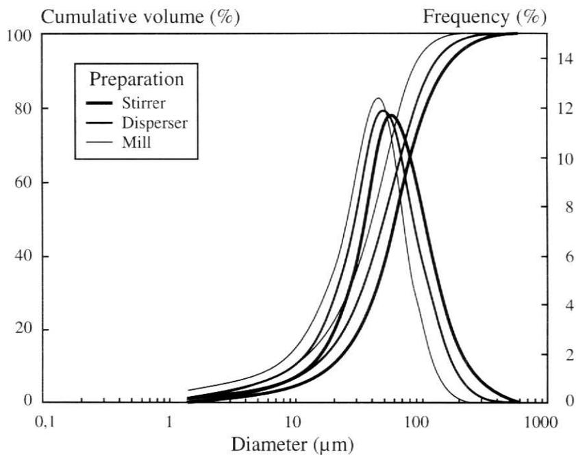
**Figure 8.** Ink L4 particle-size distribution with different preparation systems.
