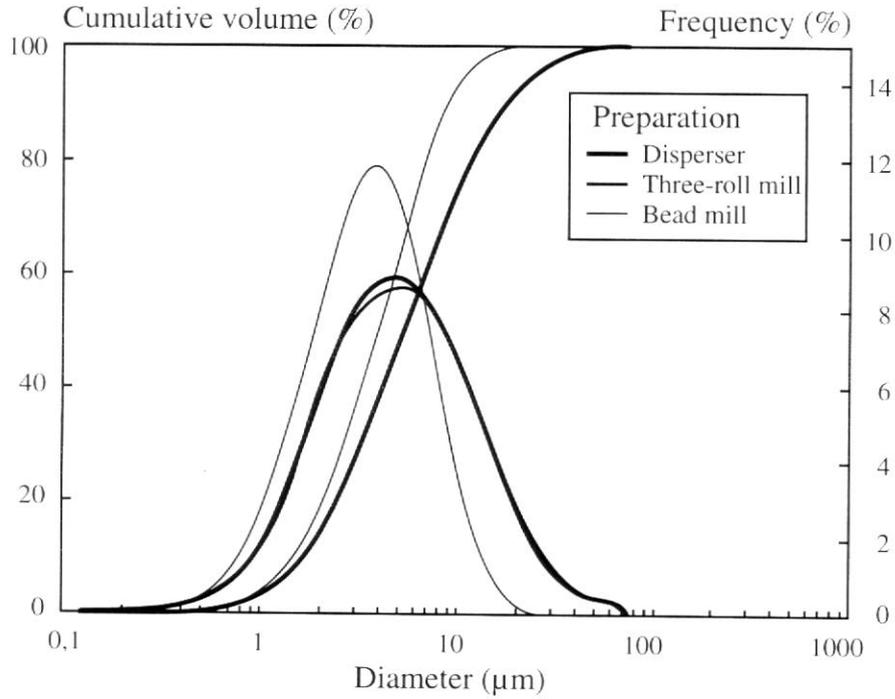
**Figure 14.** Ink I1 particle-size distribution with different preparation systems.
