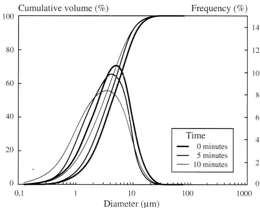
Figure 6. Effect of applying ultrasonics on a partially dispersed ink.
