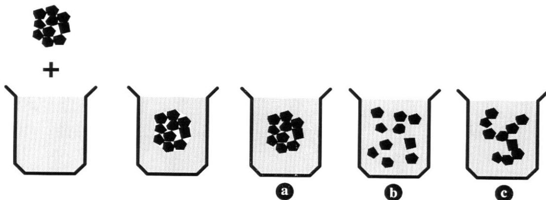
**Figure 3.** Solids dispersion stages: (a) wetting, (b) agglomerate breakup, (c) stabilization.
