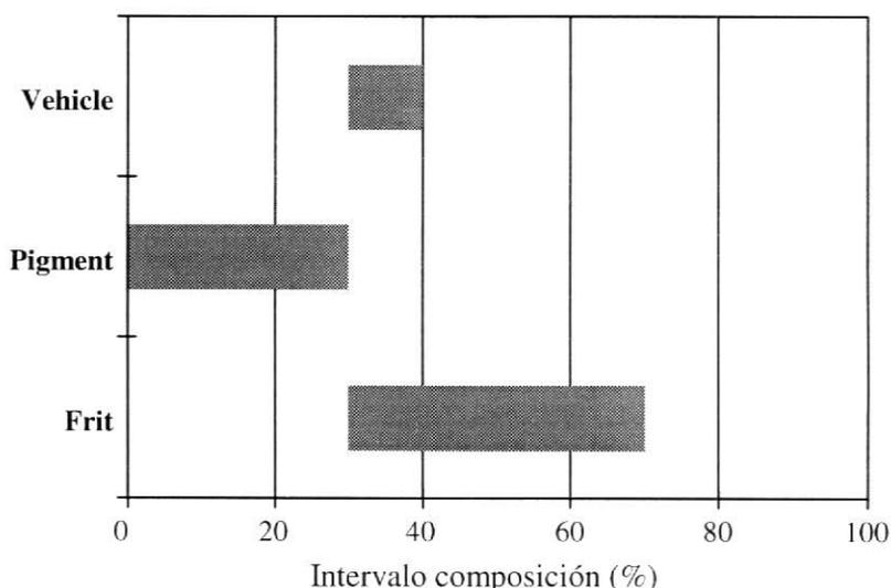
**Figure 1.** Composition interval of industrial screen-printing inks
