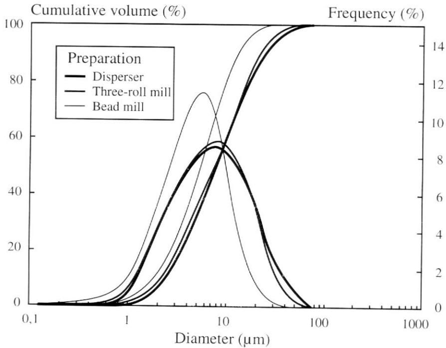
**Figure 15.** Ink I2 particle-size distribution with different preparation systems.
