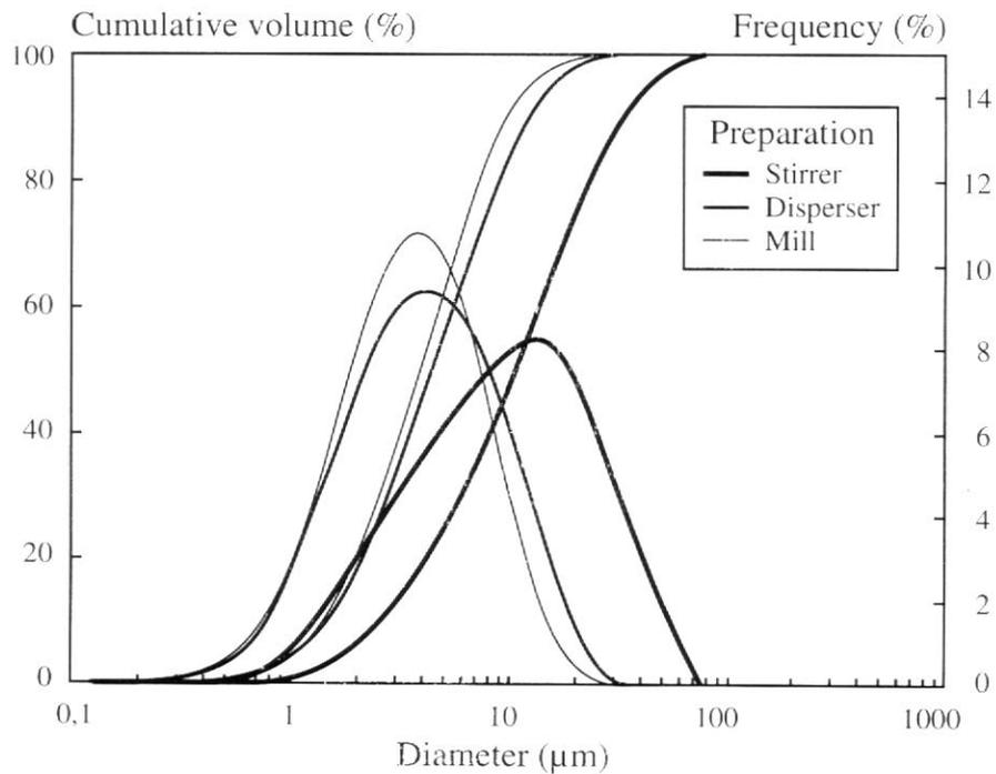
**Figure 7.** Ink L2 particle-size distribution with different preparation systems.
