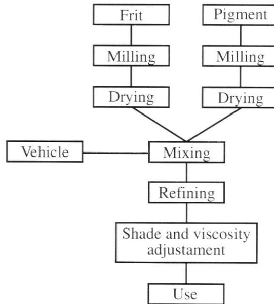
**Figure 2.** General preparation process for screen-printing inks.
