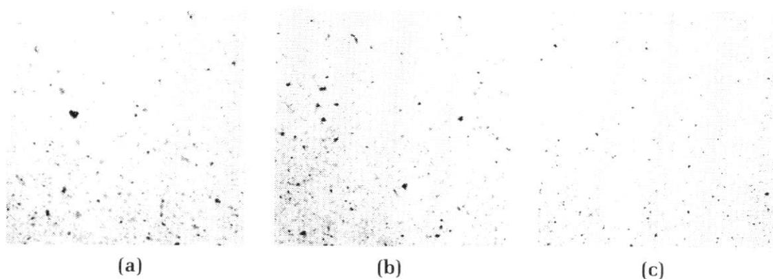
**Figure 10.** Photographs taken with an optical microscope of the screen-printed surface using ink L2, with different preparation methods: (a) stirrer, (b) disperser, (c) bead mill.
