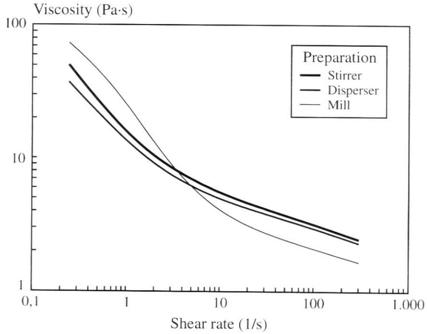
**Figure 11.** Ink L2 viscosity curve with different preparation systems.
