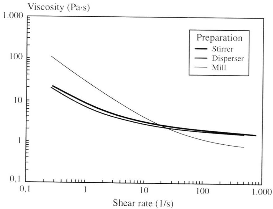
**Figure 12.** Ink L3 viscosity curve with different preparation systems.
