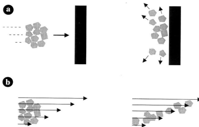
**Figure 5.** Agglomerate breakup mechanisms: (a) impact, (b) shear.
