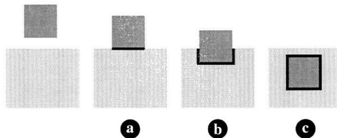
Figure 4. Stages involved in wetting a solid : (a) adhesion, (b) immersion, (c) spreading.
