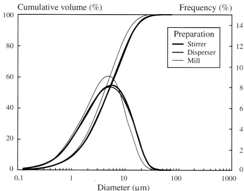
**Figure 9.** Ink L3 particle-size distribution with different preparation systems.
