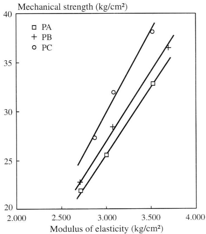
Figure 11. Relationship between mechanical strength and modulus of elasticity for different spray-dried powders.
