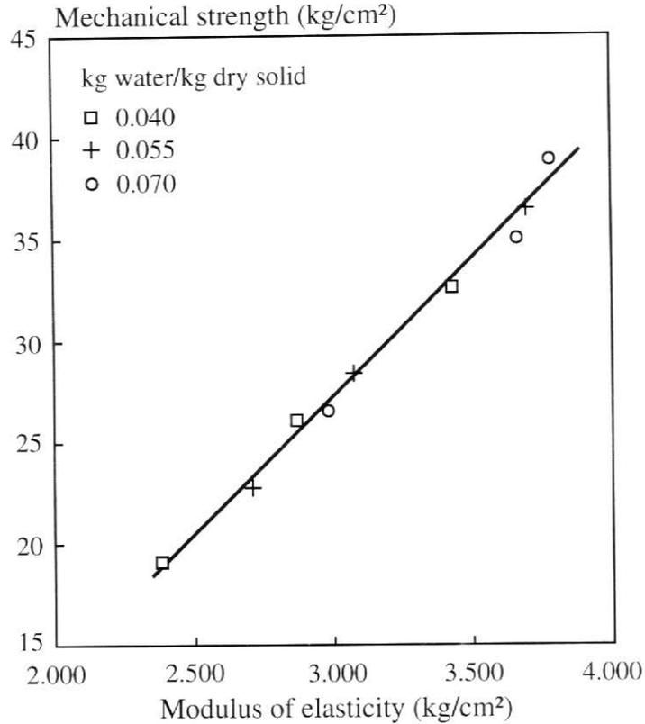
Figure 8. Relationship between dry mechanical strength and modulus of elasticity for different pressing moisture contents.
