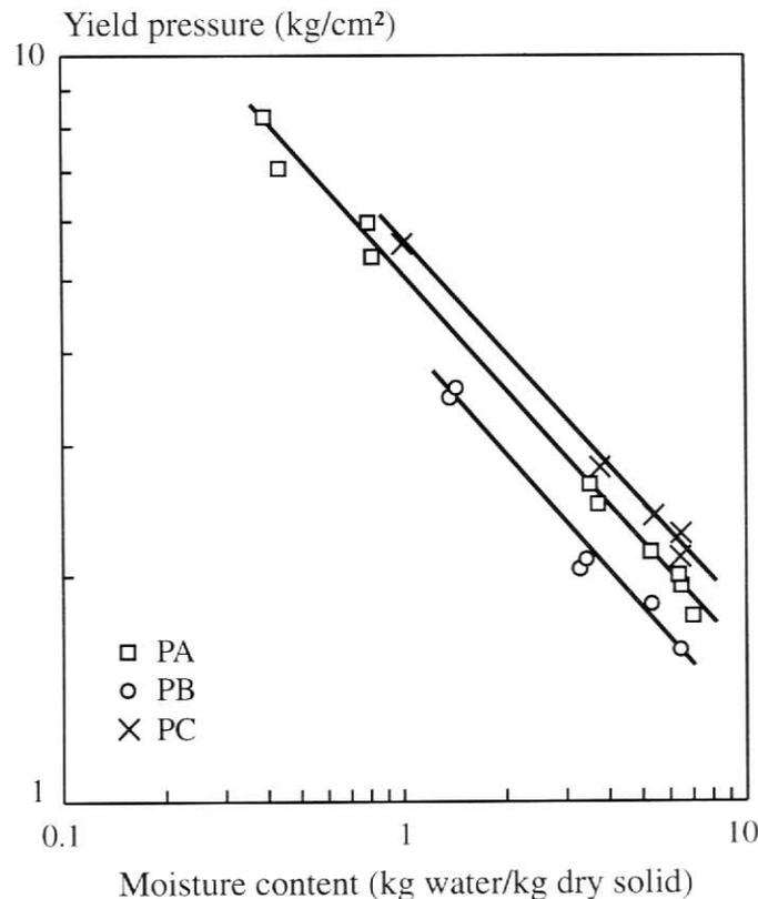
Figure 12. Variation of yield pressure with pressing moisture content for powders PA, PB and PC.
