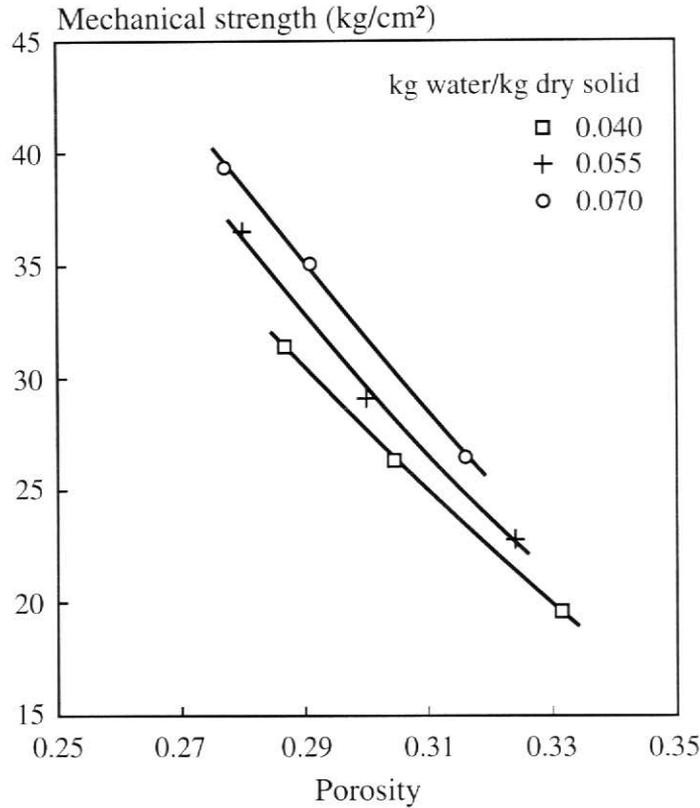
**Figure 6.** Variation of dry mechanical strength with porosity for different pressing moisture contents.
