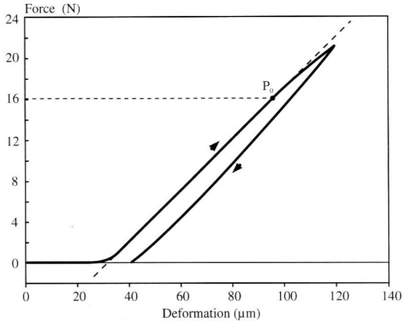
Figure 3. Load/deformation curve obtained in a cross-bending test without rupture of the sample.
