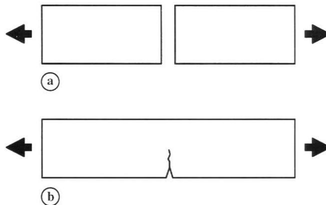
**Figure 1.** a) Rumpf's theory assumes that fracture arises simultaneously throughout the material; b) Griffith's theory assumes that rupture occurs as a result of crack propagation.
