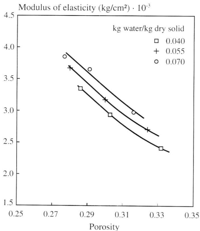
**Figure 7.** Variation of the modulus of elasticity with porosity for different pressing moisture contents.
