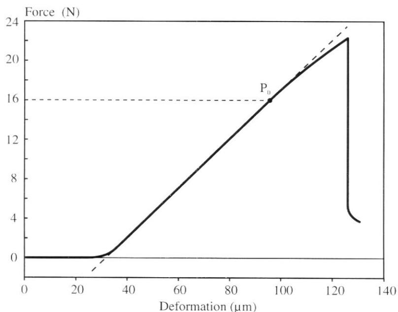
**Figure 2.** Load/deformation curve obtained in a cross-bending test with rupture of the sample.
