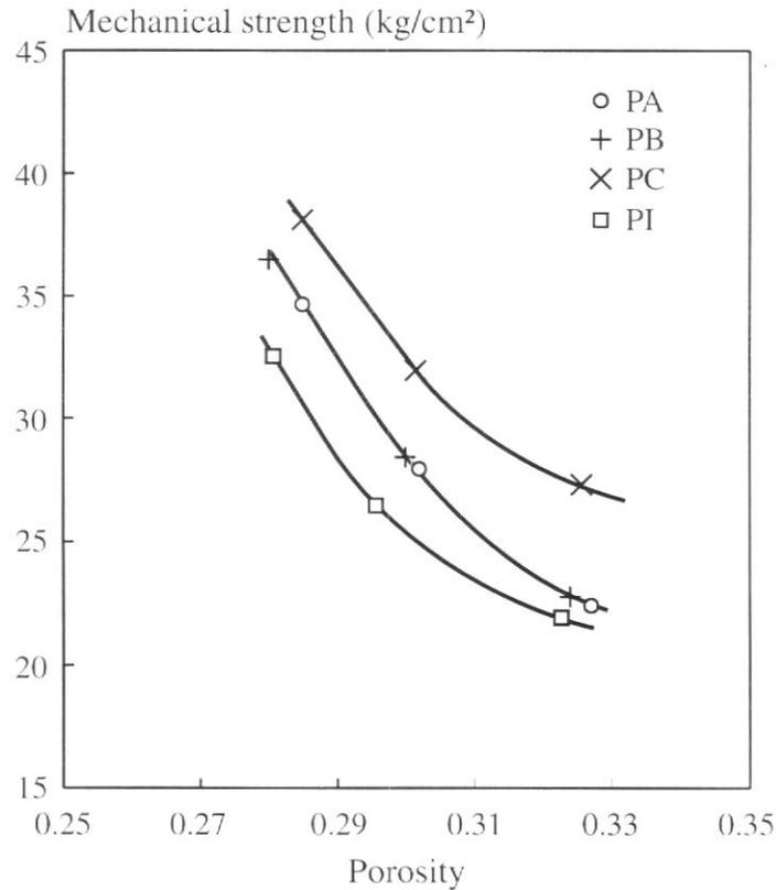
**Figure 9.** Variation of dry mechanical strength with porosity for different spray-dried powders.
