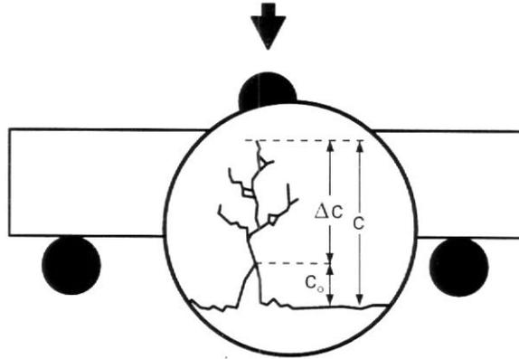
**Figure 5.** Fracture mechanism proposed for green ceramic materials.
