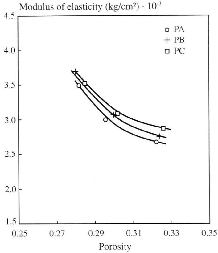
Figure 10. Variation of the modulus of elasticity with porosity for different spray-dried powders.
