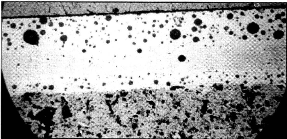
Figure 2 - Cross section of a glazed tile: porosity in the thickness of the glaze.
