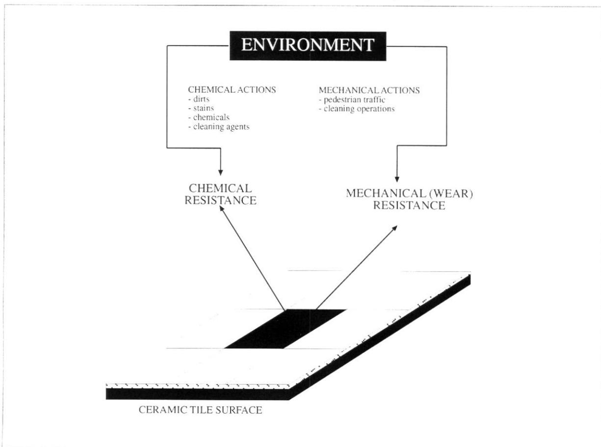
Figure 1 - Working conditions and surface performance characteristics of ceramic tiles.
