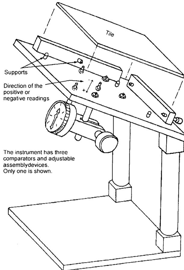
*Figure 2. Apparatus for measuring surface flatness (EN 98)*
