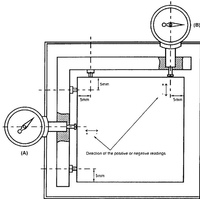
*Figure 1. Apparatus for measuring straightness of sides and rectangularity (EN 98)*
