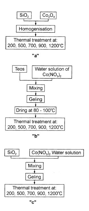
Figure 1. "a", "b", "c": Three variants for obtaining of cobaltous silicate
