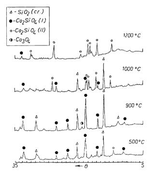
Figura 3. Diffractograms of the samples obtained dy sol-gel method version (b)
