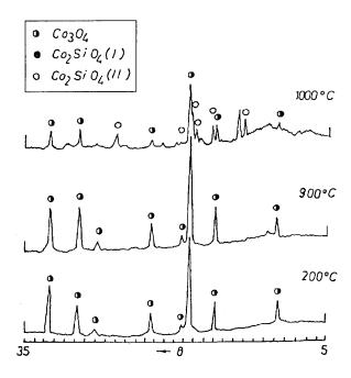
Figura 4. Diffractograms of the samples obtained by sol-gel method version (c)
