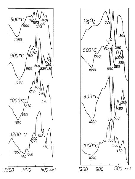
Figura 7. Ir-spectra of the gels obtained by sol-gel method (version b)
