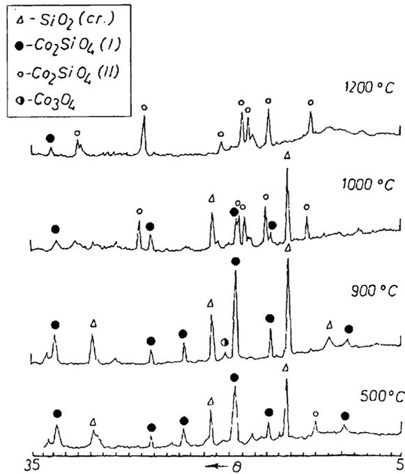
Figura 3. Diffractograms of the samples obtained by sol-gel method version (b)
