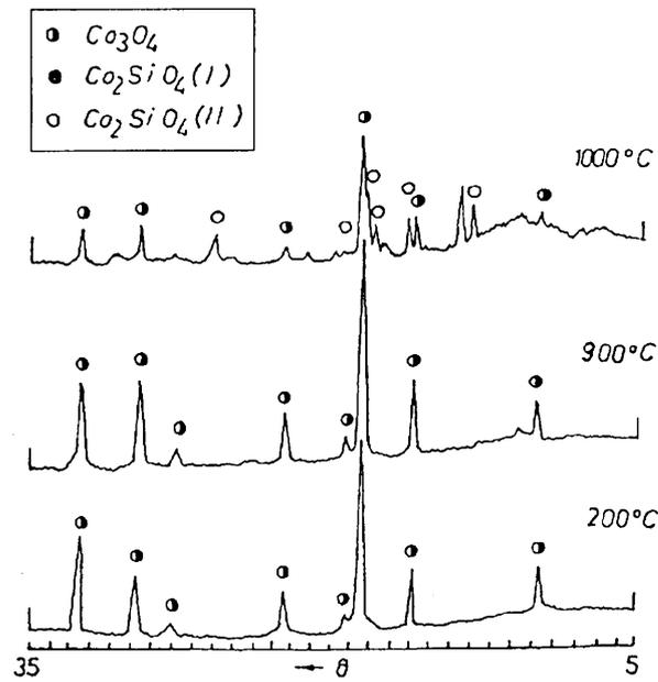
**Figura 4.** *Diffractograms of the samples obtained by sol-gel method version (c)*
