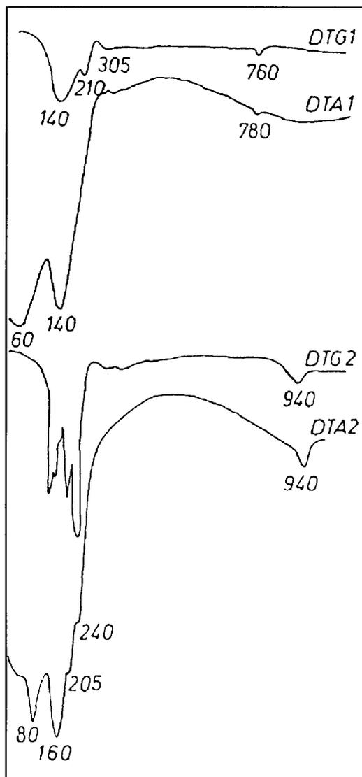
*Figura 6. DTA curvs of gels obtained by sol-gel method (version b, c)*
