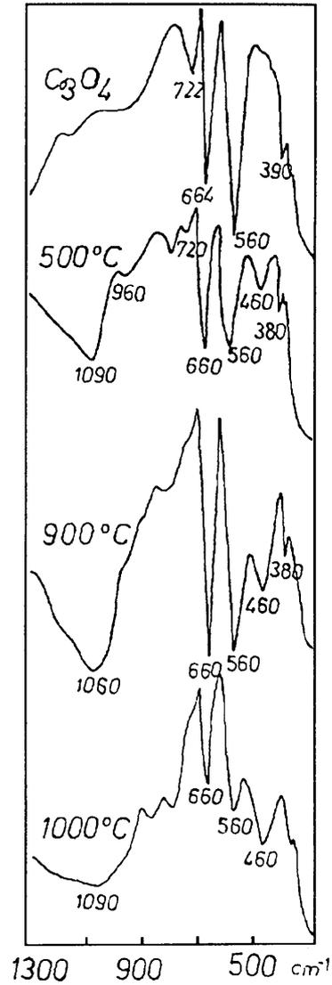
**Figura 7.** *Ir-spectra of the gels obtained by sol-gel method (version b)*
