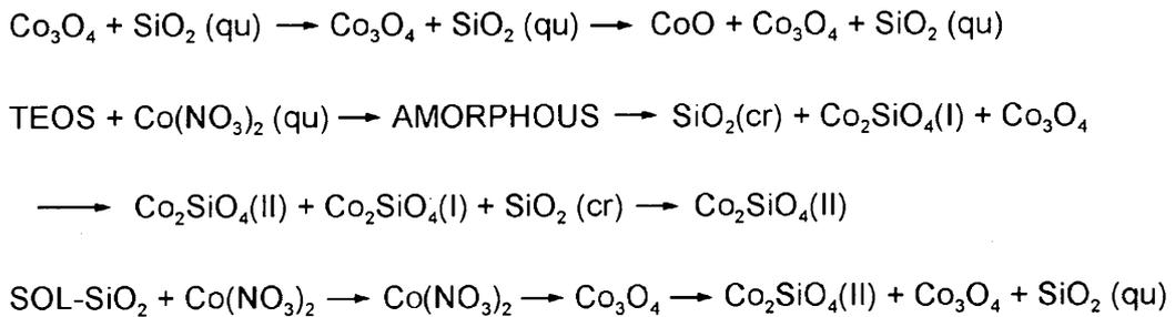
**Figura 5.** *The phaseforming mechanism related to the temperature increasing by the three synthesis versions*
