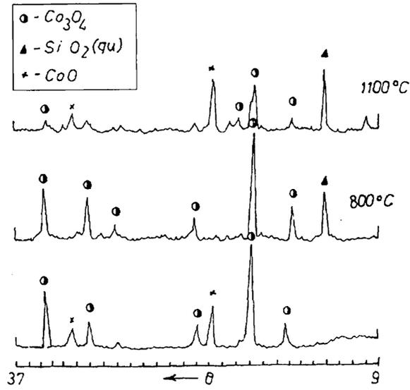
Figura 2. Diffractograms of the samples obtained by the conventional ceramic method version (a)
