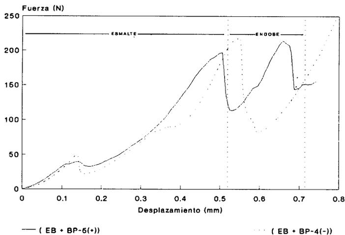
Figure 19. Effect of particle-size distribution on white glaze bonding to the EB engobe
