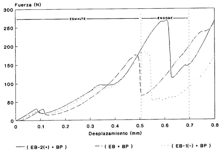
Figure 15. Bonding between the white glaze and engobes with varying bentonite contents
