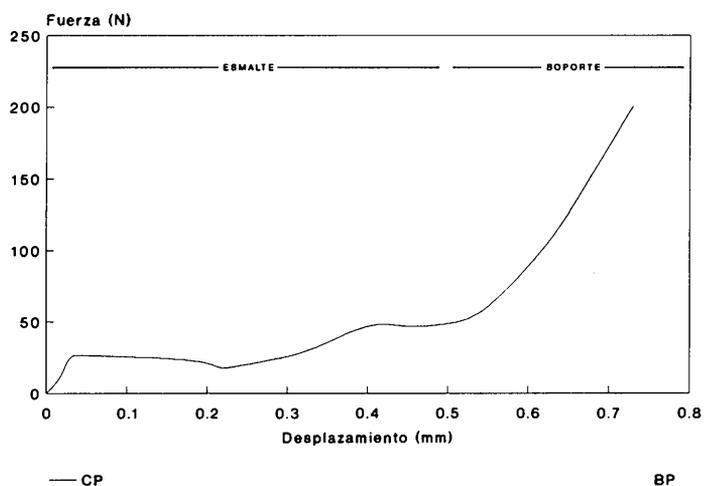
Figure 4. CP crystalline glaze and BP white glaze bond
