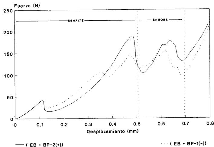
Figure 16. Bonding of white glazes BP-1 and BP-2 with differing binder contents to engobe EB
