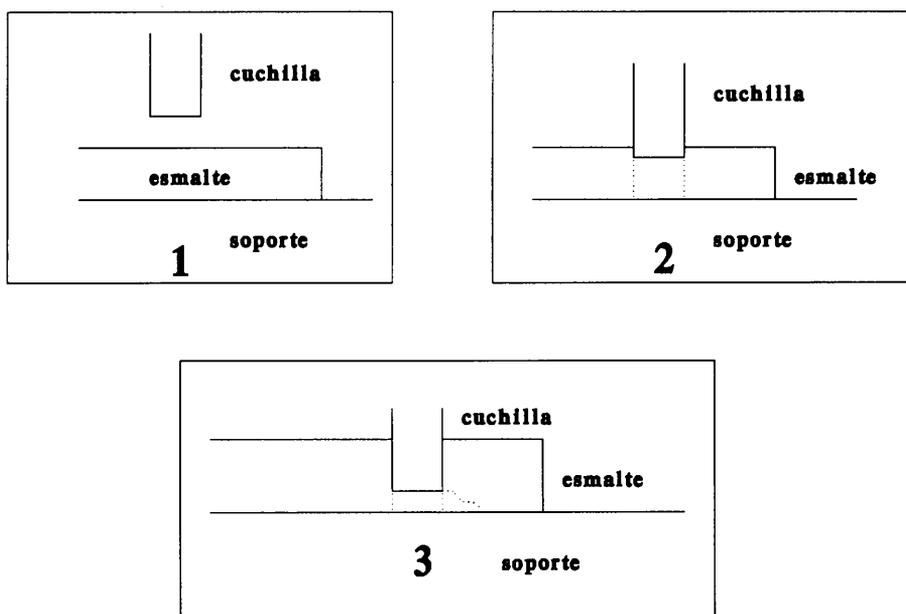
Figure 2. Schematic of layer fracture
