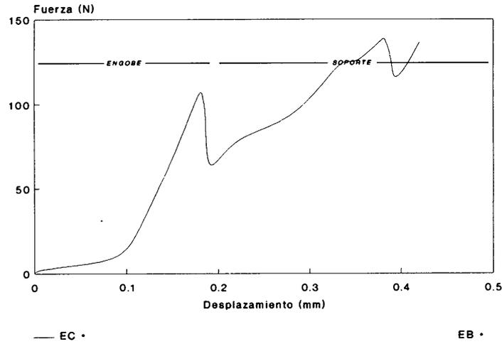
Figure 5. EC and EB engobe layer bond obtained from the corresponding aged suspensions
