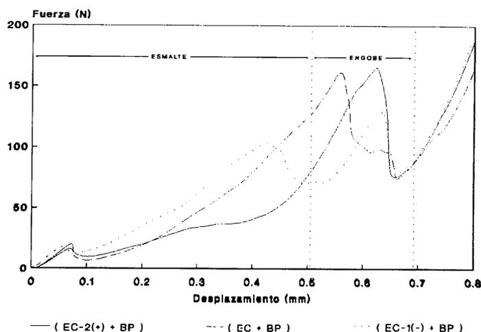
Figure 14. Bonding between the white glaze and engobes with varying organic binder content
