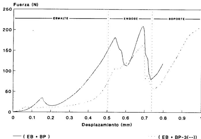
Figure 17. Bonding of white glazes BP and BP-3 with differing binder contents to engobe EB
