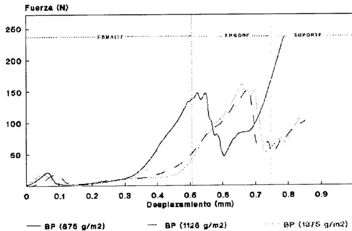
Figure 20. Glaze BP and engobe EB bond with varying amounts of applied glaze
