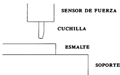
Figure 1. Schematic of the experimental assembly used
