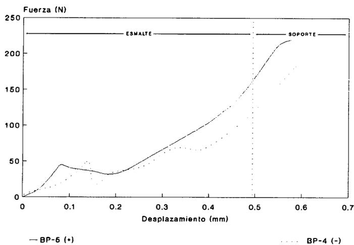
Figure 18. Effect of particle-size distribution on the white glaze bond
