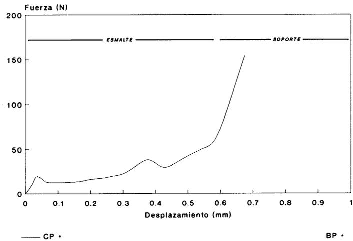
Figure 6. CP and BP glaze layer bond obtained from the corresponding aged suspensions
