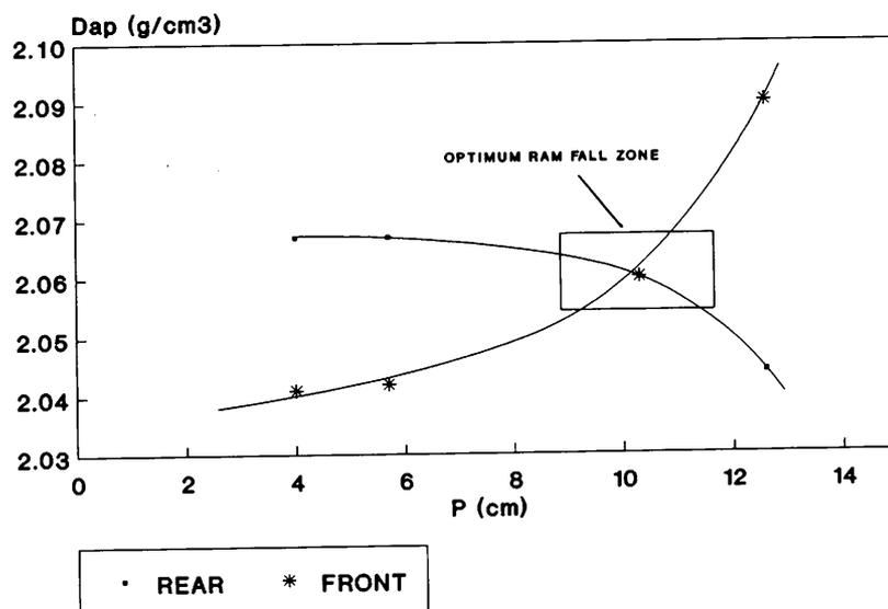
Figure 11. Bulk density of the front and rear zones in function of the fall point of the lower ram.
