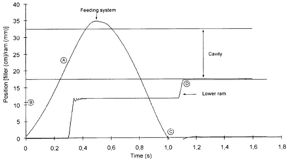
**Figure 7.** Filler and ram positions during filling.
