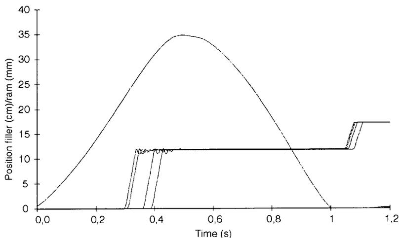
Figure 8. Position of the lower ram and feeding system in the manoeuvres performed.
