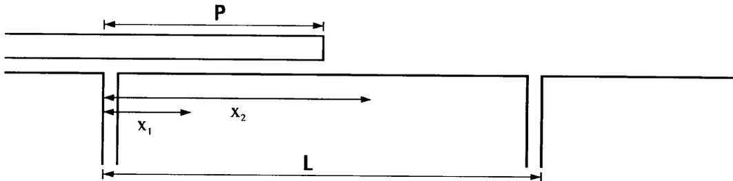
Figure 9. Schematic of cavity filling.
