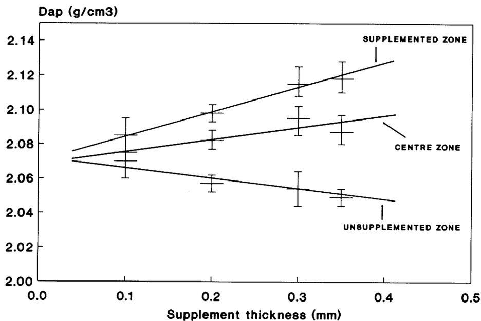
Figure 14. Compaction variation in each zone in function of the thickness of the supplement used.
