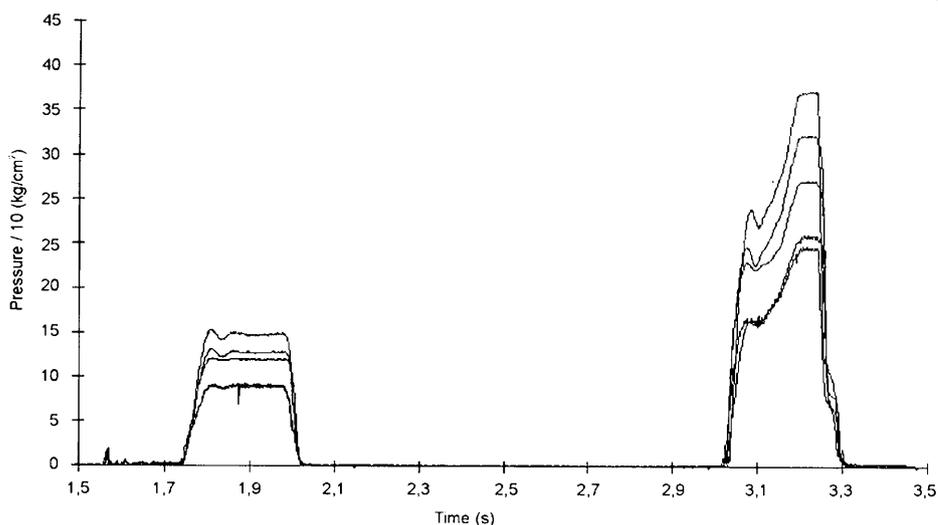
Figure 12. Pressure distribution in the piece travelling a compression cycle
