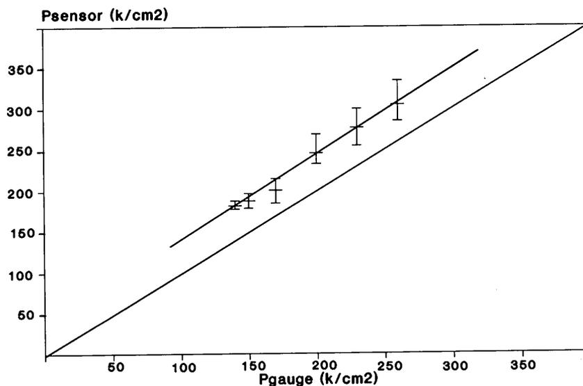
Figure 15. Maximum gauge pressure versus sensor-measured maximum pressure.
