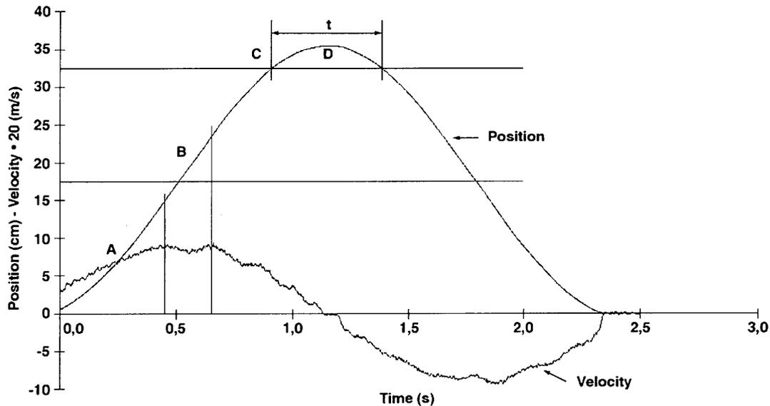
Figure 2. Position and velocity of the filler during charging of the cavity.
