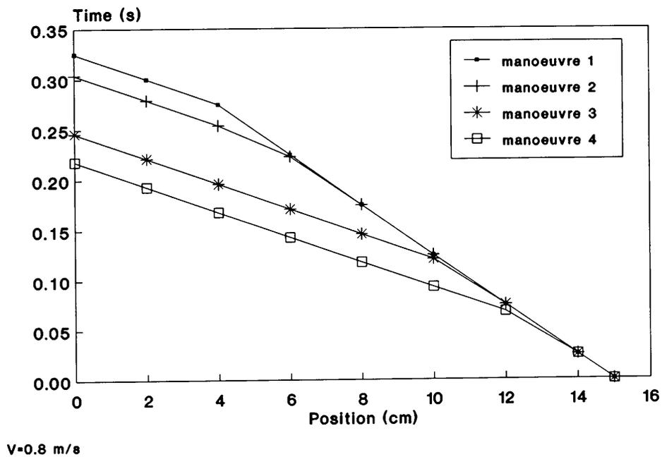
Figure 10. Dwell times of the feeding system over the cavity, in function of its position over it, for each manoeuvre.
