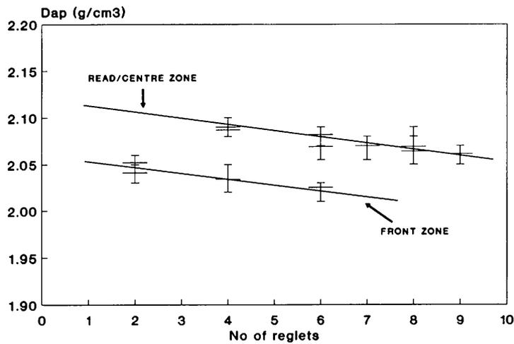
**Figure 4.** Bulk density in each zone of the piece in function of the number of reglets crossing it.
