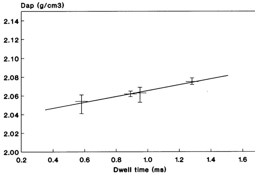
**Figure 6.** Effect of filler dwell time over the cavity on overall bulk density of the piece.
