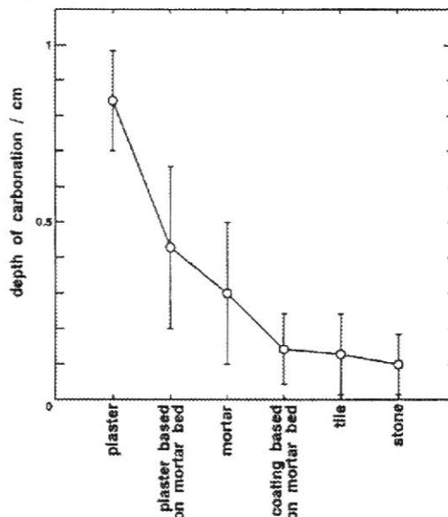
**Fig.6** The results of survey regarding the effect of exterior tiles on the inhibition of carbonation of concrete.
