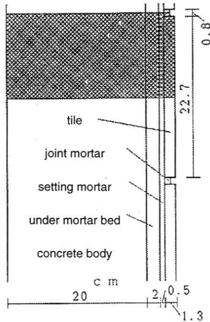
Fig.8 The section model of the tile shielding wall for FEM analysis
