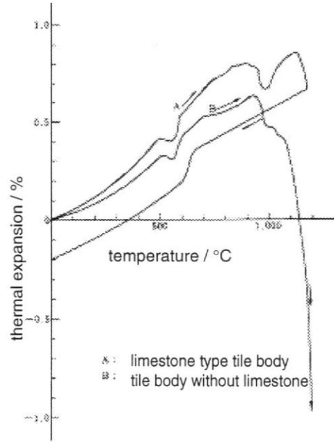
**Fig.5** The thermal expansion curves of tile bodies with and without limestone addition
