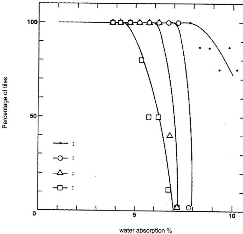
**Fig.3** Percentage of interior tiles that survive the freeze/thaw test and the results of outdoor exposure test.
