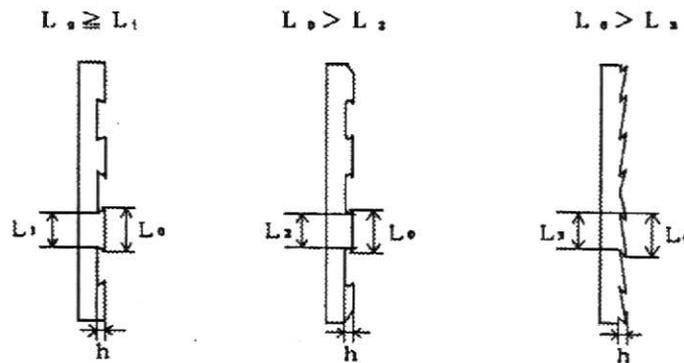
Table 1. Standard of the grooves in the back surfaces of exterior tiles(JIS A-5209)
