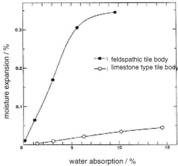
**Fig.4** Moisture expansion behavior of feldspathic tile body and limestone type tile body
