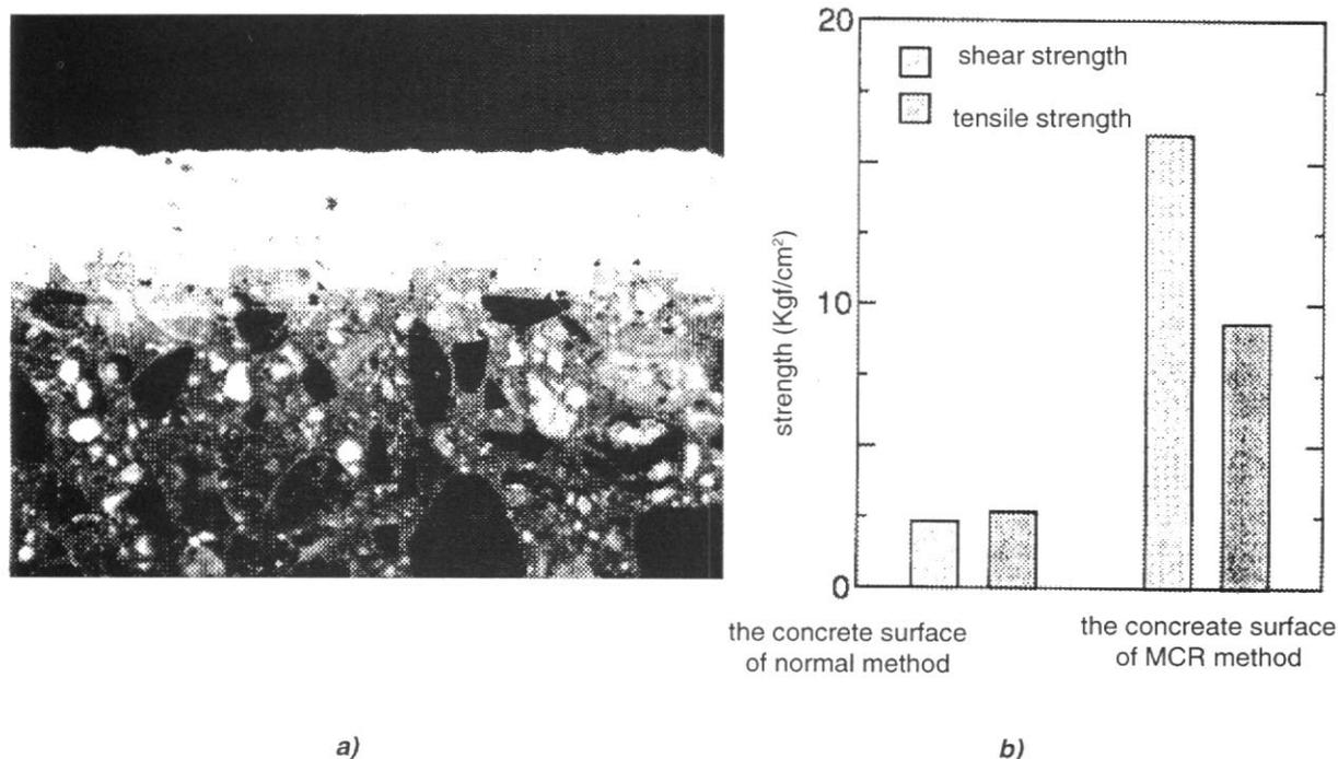
**Fig.7** a) *The interface between concrete and mortar in the MCR method*
