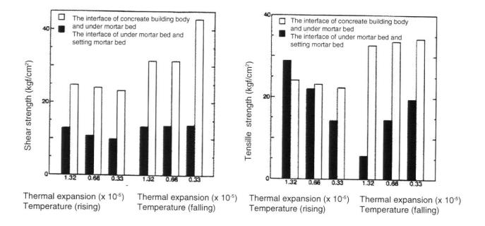
Fig.9 The shearing and tensile strengths calculated with respect to the coefficient of thermal expansion of the tile.
