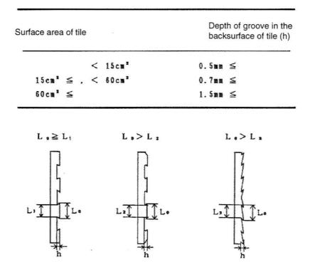
Table 1. Standard of the grooves in the back surfaces of exterior tiles(JIS A-5209)
