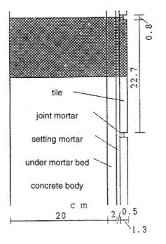
Fig.8 The section model of the tile shielding wall for FEM analysis
