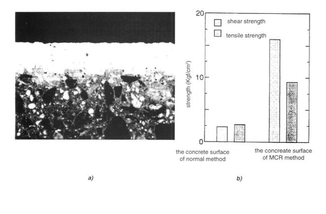
Fig.7 a) The interface between concrete and mortar in the MCR method b) The results of shearing and tensile tests carried out after curing
