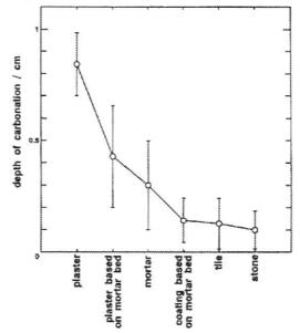
Fig.6 The results of survey regarding the effect of exterior tiles on the inhibition of carbonation of concrete.
