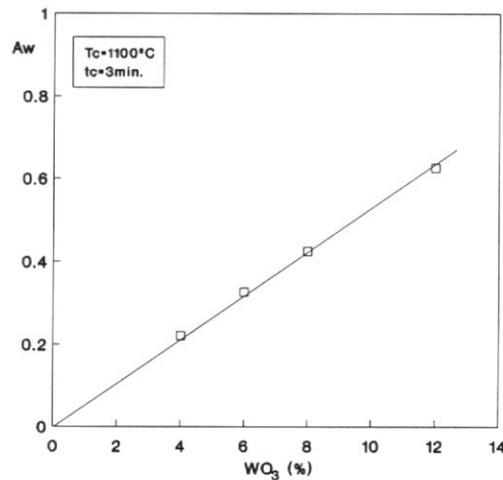
Figure 5. Relationship between the surface fraction occupied by crystalline phases ( $A_w$ ) and the  $WO_3$  content in the screen print.
