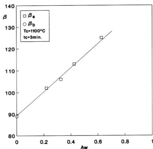
Figure 6. Relationship between screen-printed surface gloss ( $\beta_s$ ) and the surface fraction occupied by crystals ( $A_w$ ). Base glaze gloss:  $\beta_b$ .
