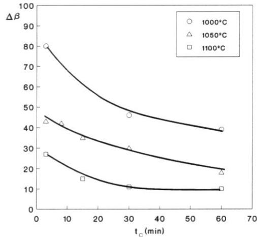
**Figure 11.** Influence of maximum firing temperature ( $T_c$ ) and dwell time at this temperature ( $t_c$ ) on the intensity of the decorative effect ( $\Delta\beta$ ).
