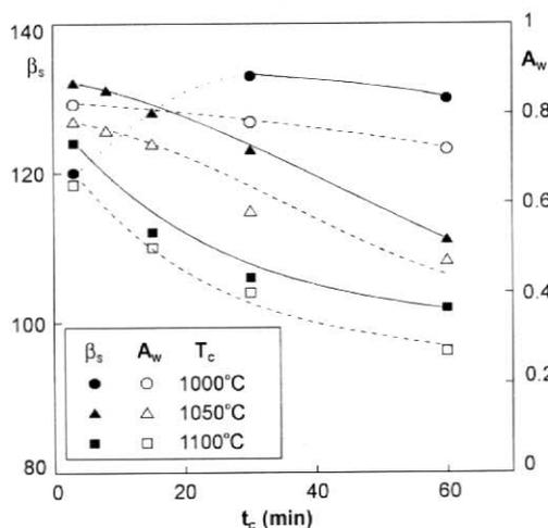
Figure 7. Influence of  $T_c$  and  $t_c$  on screen-printed surface gloss ( $\beta_s$ ) and the fraction occupied by crystals ( $A_w$ ).  $\text{WO}_3$  content = 8%
