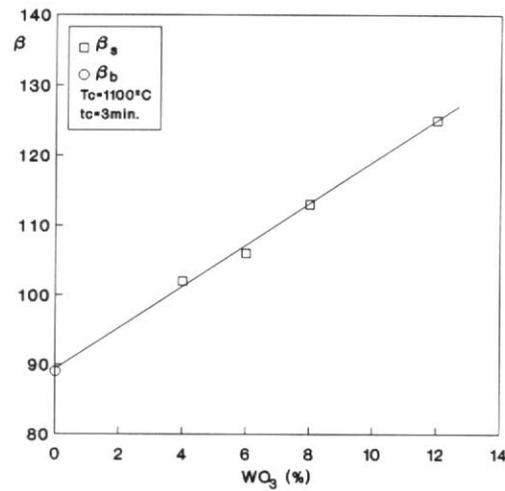
Figure 4. Variation of screen-printed surface gloss ( $\beta_s$ ) with  $WO_3$  content. Base glaze gloss:  $\beta_b$ .
