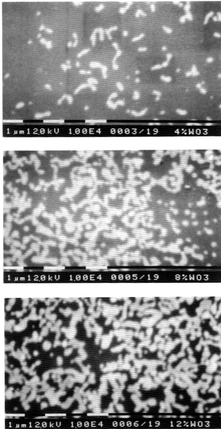
**Figure 2.** Effect of  $WO_3$  content in the screen-printing paste on microstructure of the resulting surface ( $T_c=1100^\circ\text{C}$ ;  $t_c=3$  min)
