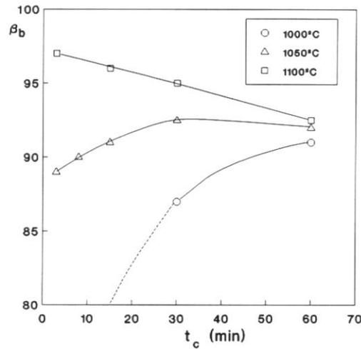
**Figure 8.** Influence of maximum firing temperature ( $T_c$ ) and dwell time at this temperature ( $t_c$ ) on base glaze gloss ( $\beta_b$ ).
