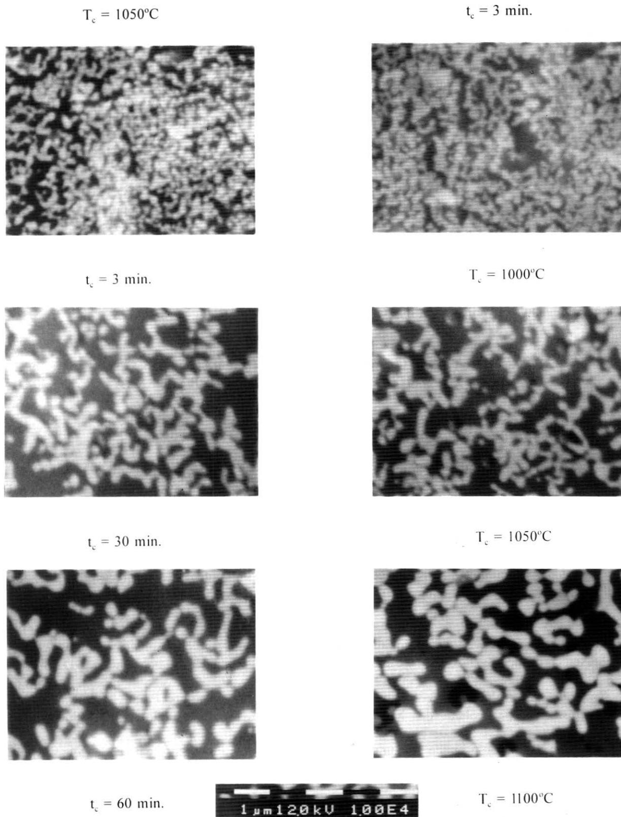
**Figure 3.** Influence of maximum firing temperature ( $T_c$ ) and dwell time at this temperature ( $t_c$ ) on microstructure of the resulting screen-printed surface.  $\text{WO}_3$  content = 8%
