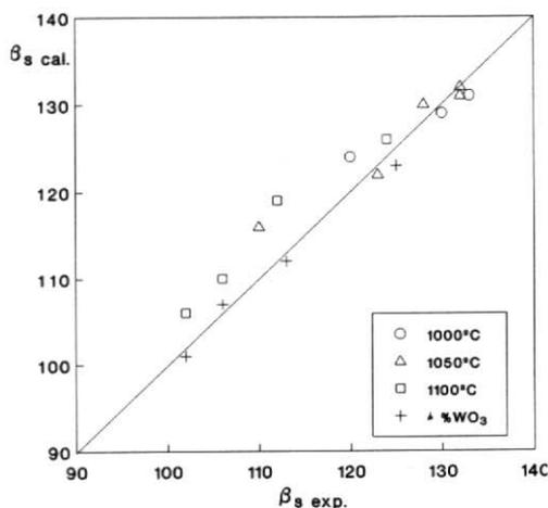
Figure 10. Comparison between the experimental results and those calculated by Equation (2).
