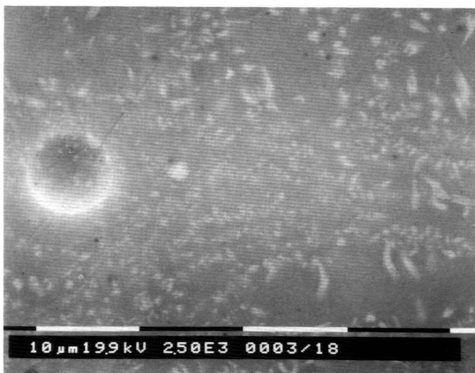
*Figure 6. Photograph of the microstructure of the glaze fired at a maximum temperature of 1000°C.*
