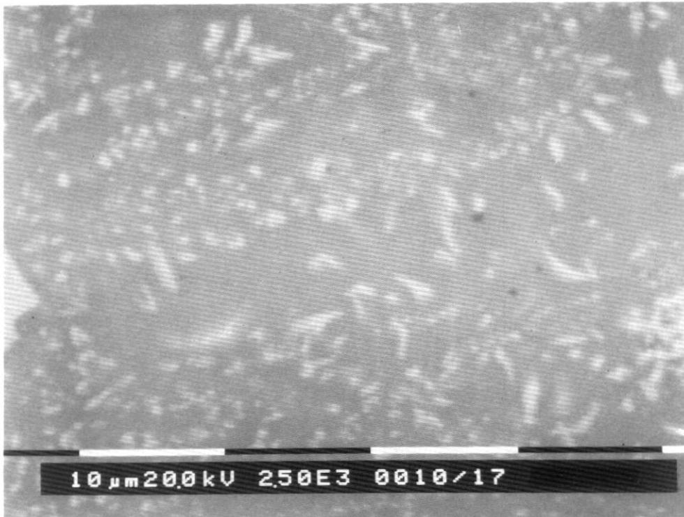
*Figure 7. Photograph of the microstructure of the glaze fired at a maximum temperature of 1050°C.*
