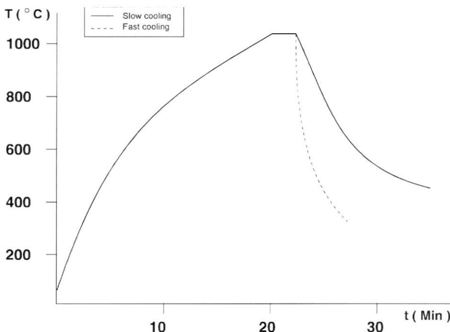
Figure 1. Firing cycles used.
