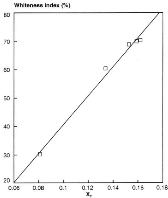
Figure 10. Variation of the whiteness index of the glaze with its crystallized zircon fraction.
