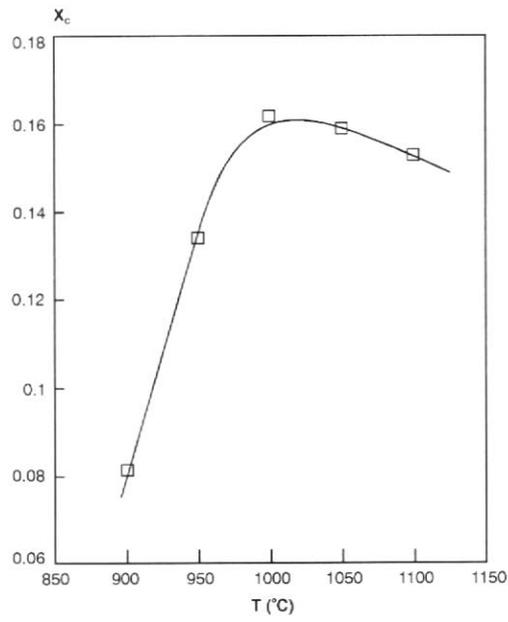
**Figure 3.** Influence of firing cycle maximum temperature upon the crystallized zircon fraction in the resulting glaze.
