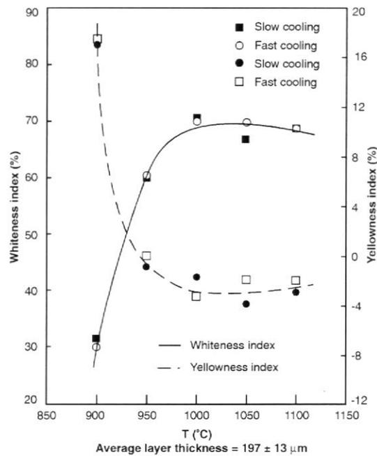
**Figure 2.** Variation of the whiteness and yellowness indexes with maximum firing temperature, in the firing cycles used
