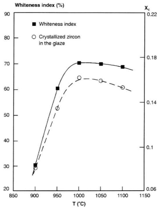
Figure 9. Variation of the whiteness index of the glaze and its crystallized zircon fraction with maximum firing temperature
