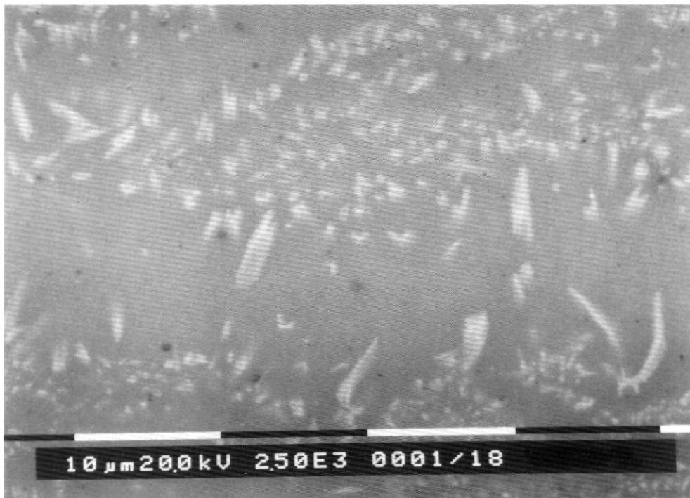
*Figure 8. Photograph of the microstructure of the glaze fired at a maximum temperature of 1100°C.*
