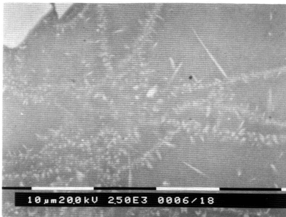
*Figure 5. Photograph of the microstructure of the glaze fired at a maximum temperature of 950°C.*
