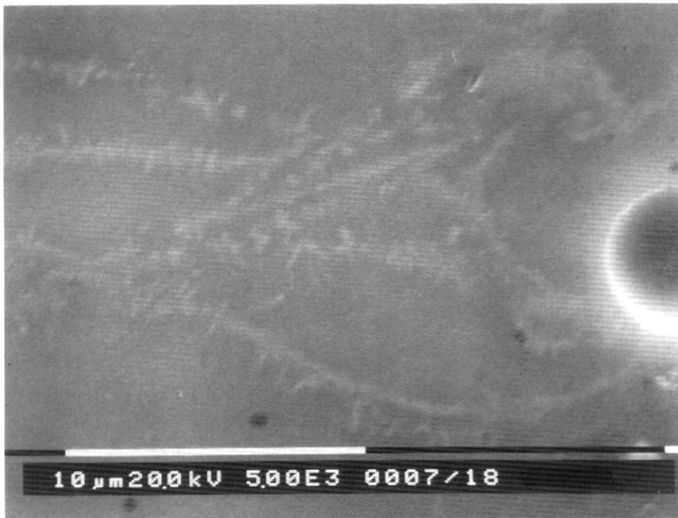
**Figure 4.** Photograph of the microstructure of the glaze fired at a maximum temperature of 900°C.
