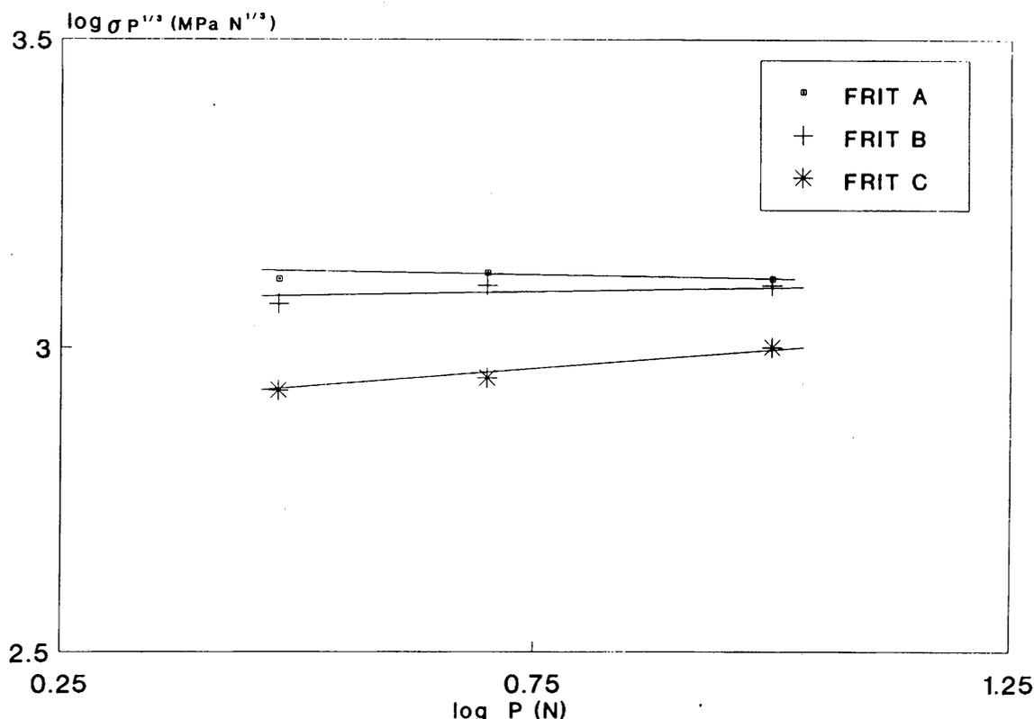
Figure 5. Relation between the product  $\sigma P^{1/3}$  and the indenter load.
