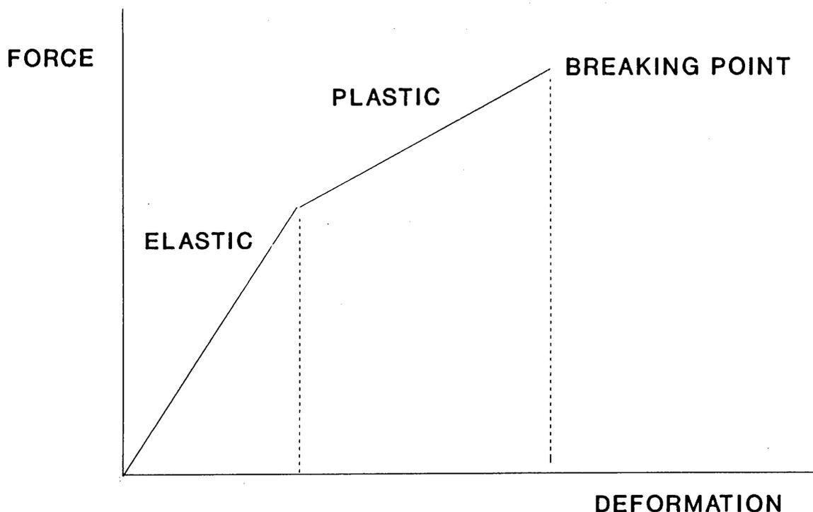
Figure 1. Mechanical behaviour of a solid.
