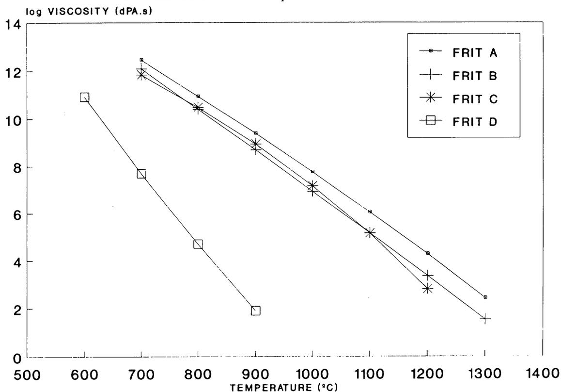
Figure 2. Viscosity-temperature curves.
