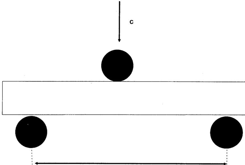
Figure 4. Scheme representing the position of the piece in the cross-bending test.
