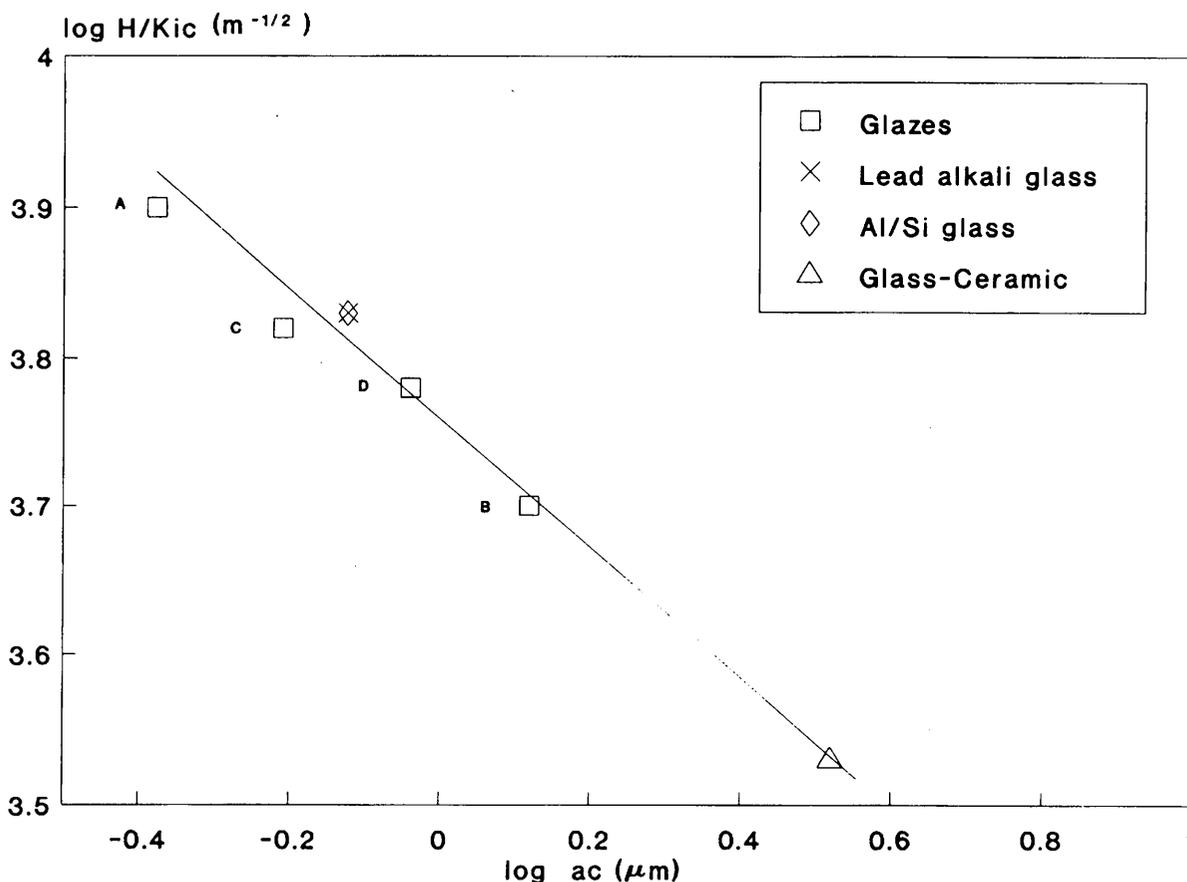
Figure 6. Relation between the ratio  $(H/K_{Ic})$  and  $a_c$ .
