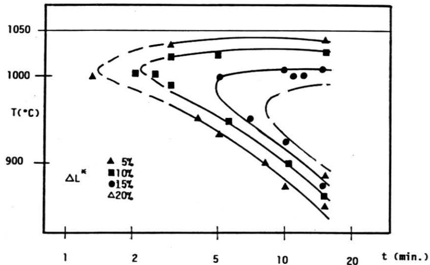
Figure 21. Curves of the same whiteness index values ( $\Delta L^*$ ) obtained from isothermal treatment.
