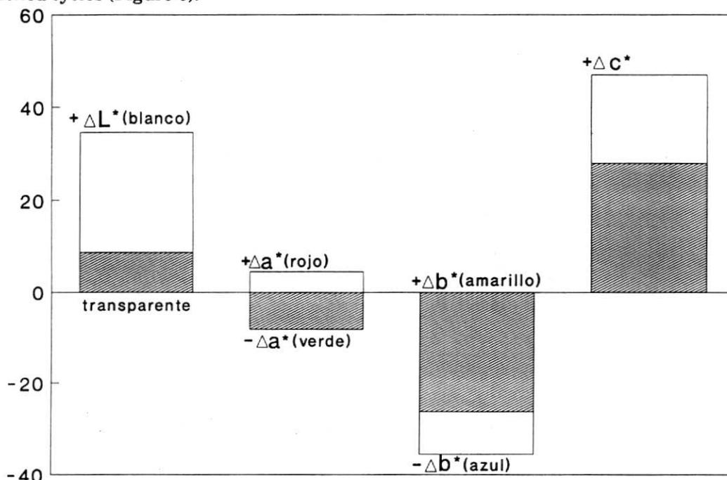
Figure 9. Colour difference ( $\Delta C^*$ ) and chromatic coordinates ( $\Delta L^*$ ,  $\Delta b^*$  and  $\Delta a^*$ ) between the glaze fired and removed from the kiln at 1100°C (virtually transparent) and the glazes after cooling by a slow cycle (type A). Cooling time from 1100 to 750°C was 25 min.
