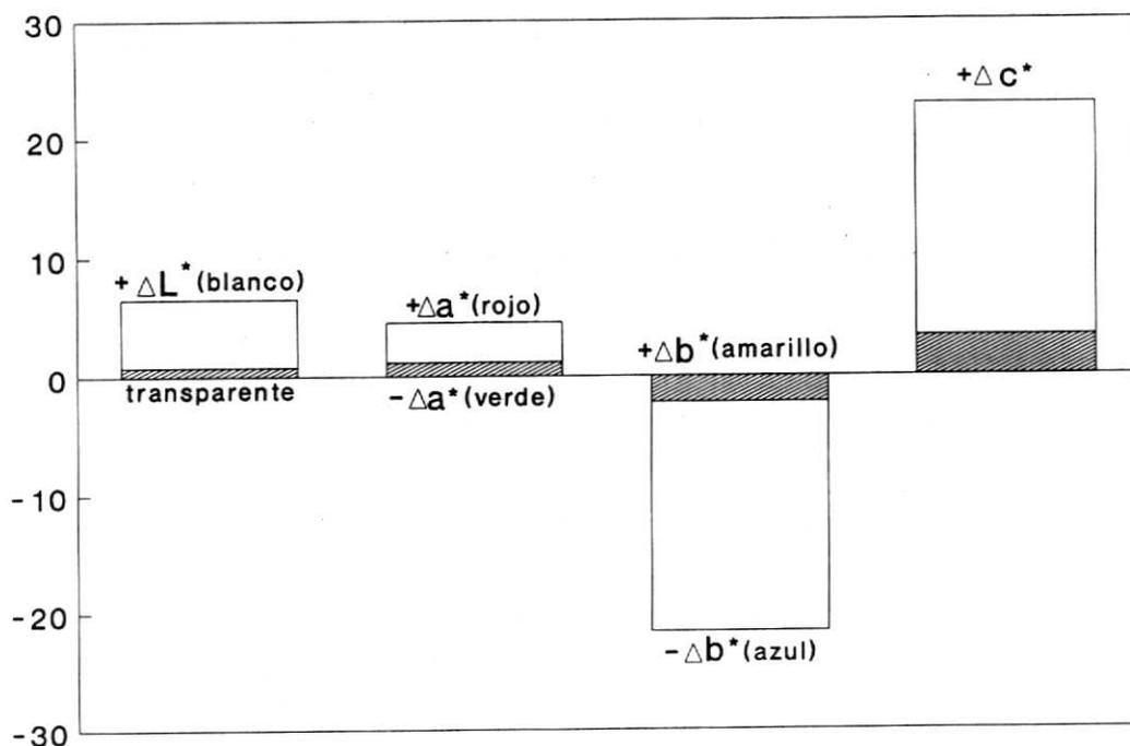
Figure 10. Colour difference ( $\Delta C^*$ ) and chromatic coordinates ( $\Delta L^*$ ,  $\Delta b^*$  and  $\Delta a^*$ ) between the glaze fired and removed from the kiln at 1100°C (virtually transparent) and the glazes after cooling by a fast cycle (type B). Cooling time from 1100 to 750°C was 3.5 min.
