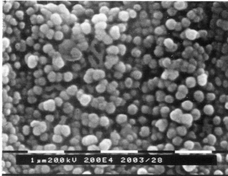
Figure 16. Microstructure of a bluish glaze.
