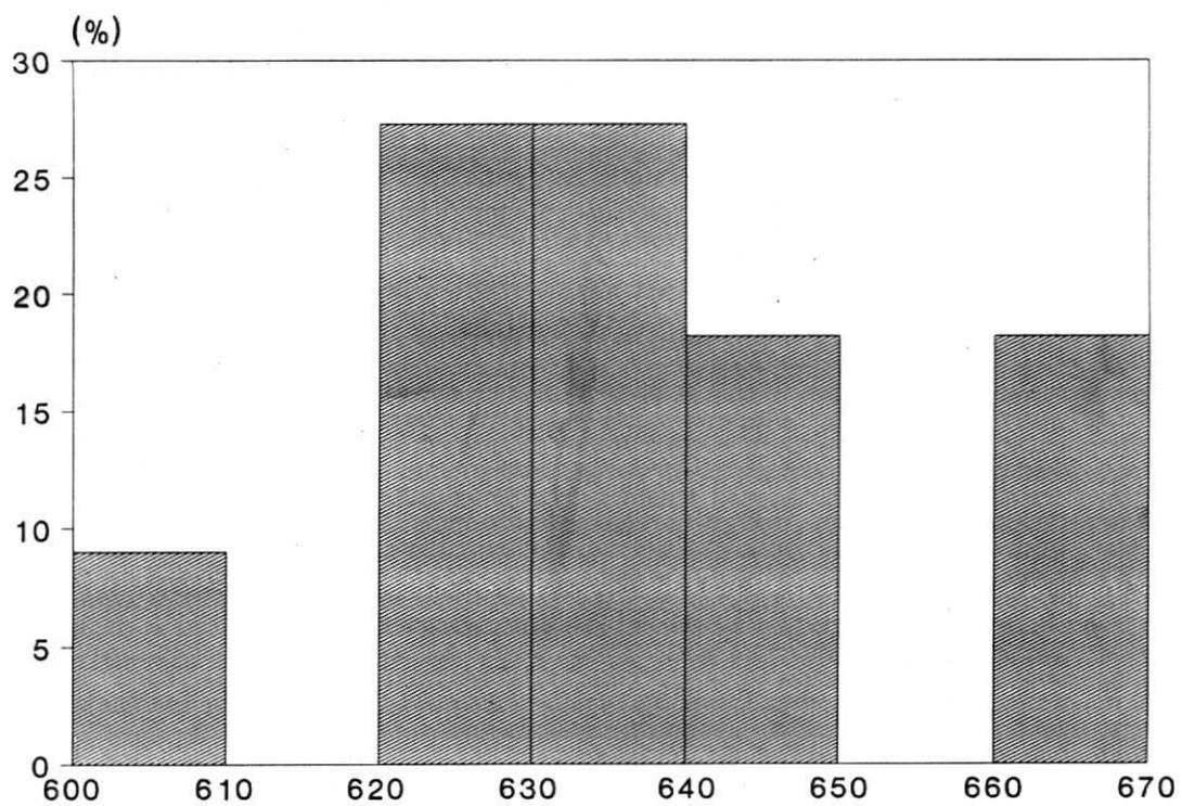
Figure 4. Transformation temperatures of the frits used.
