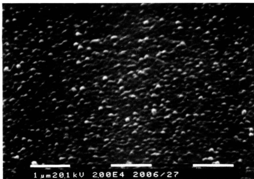
Figure 14. Microstructure of a transparent glaze.
