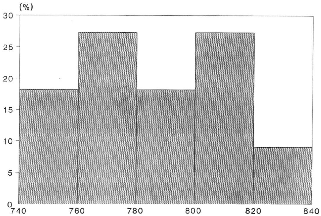
Figure 5. Softening temperatures of the frits used.
