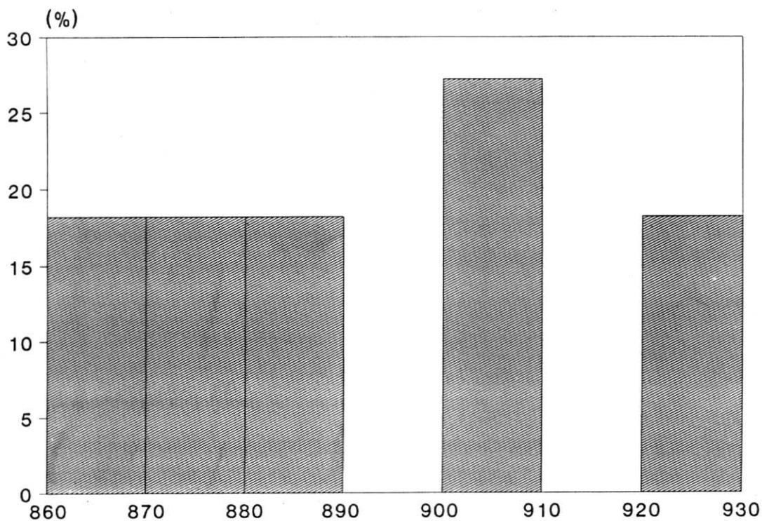
Figure 3. Sealing temperatures of the frits used.
