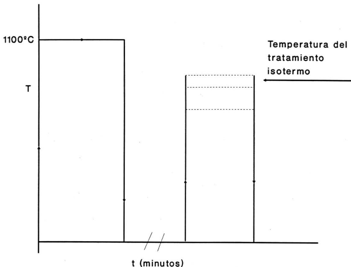
Figure 7. Isothermal treatment method to determine the rate of change in colour of the glazes.
