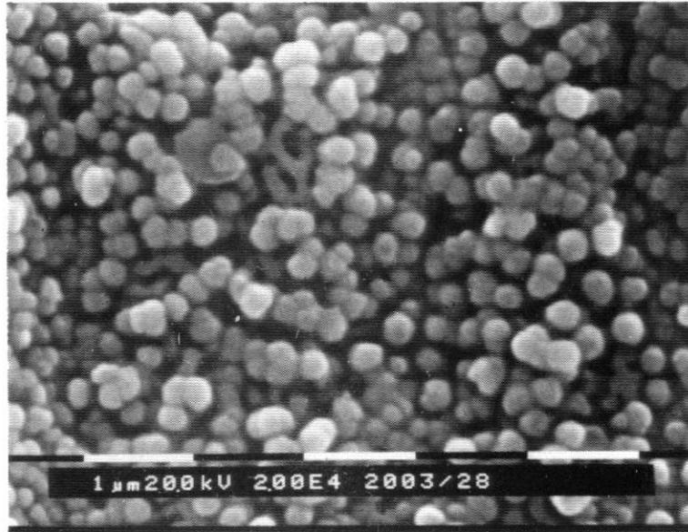
Figure 15. Microstructure of a bluish glaze.
