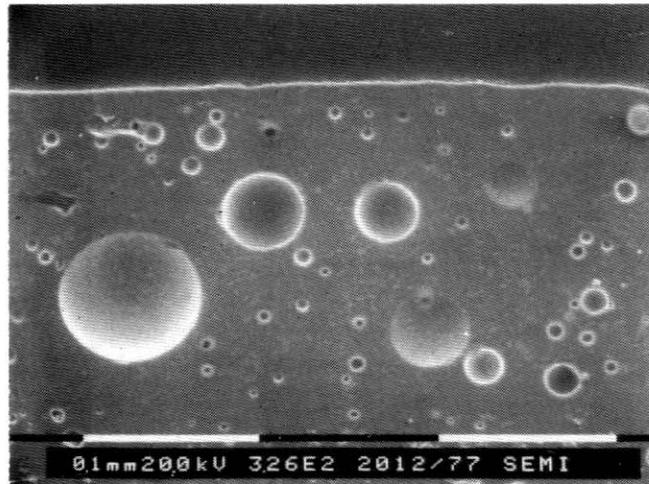
Figure 16.- SEM photograph, magnification (326x), of the cross-section of the matt glaze.
